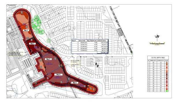
Groundwater dewatering will be implemented sequentially for each bay to drawdown the water table to a sufficient level for bulk earthworks to be undertaken. The drawdown target for construction is at least 1.0 m below the lake subgrade level, which Walker expects to be sufficient based on advice from civil contractors.
