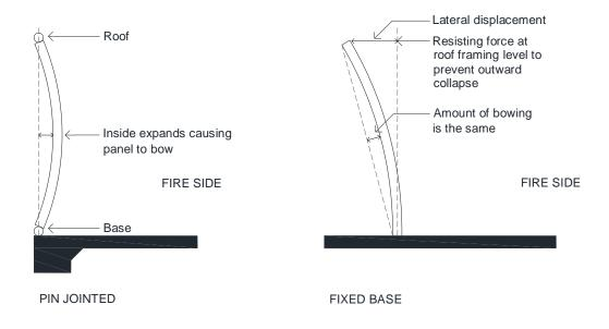
Figure 3(b) Behaviour of concrete panels exposed to fire
