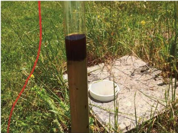
Photograph 13: Showing a grab sample from the disused septic with LNAPL sitting above liquid waste
