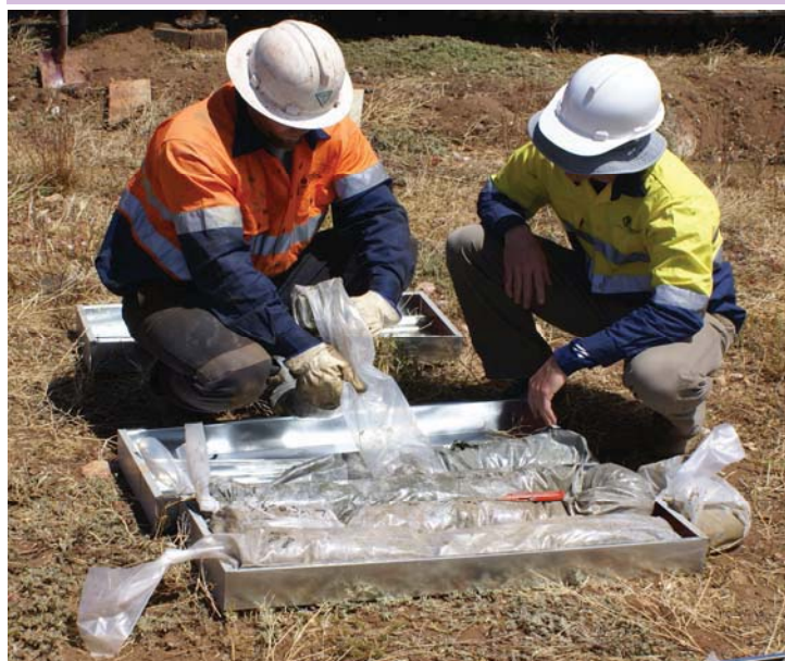
Golder Associates' geotechnical engineer reviews drill core samples with a Sonic Rig Driller at the Sheep Hill Port site.
