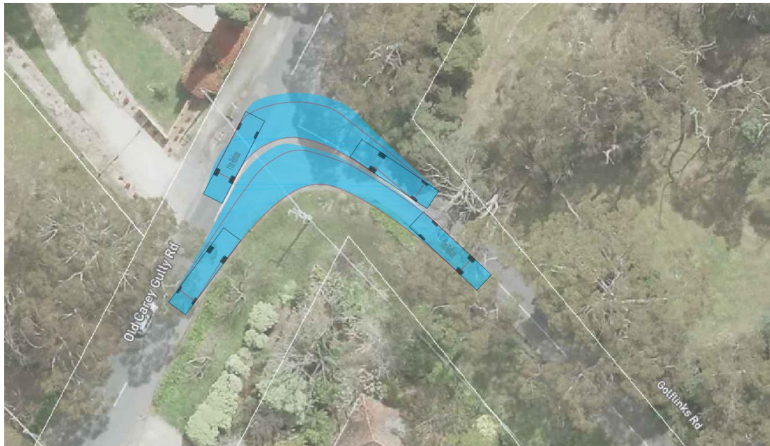
Figure 7 - Indicative commercial vehicle swept paths at the Golflinks Road/Old Carey Gully Road intersection
