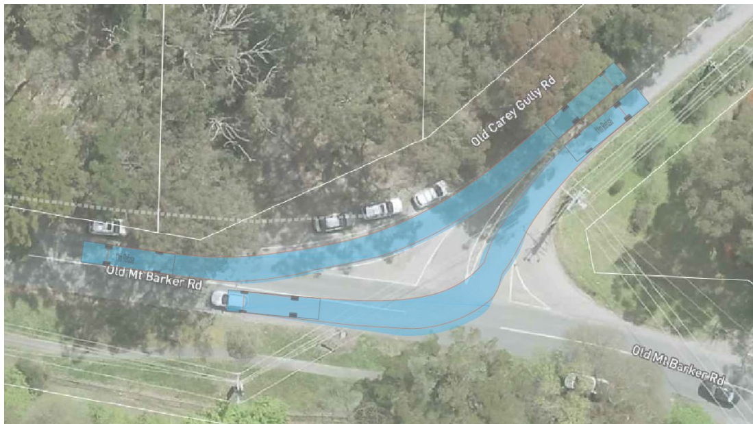
Figure 8 - Indicative commercial vehicle swept paths at the Old Carey Gully Road/Old Mount Barker Road intersection
