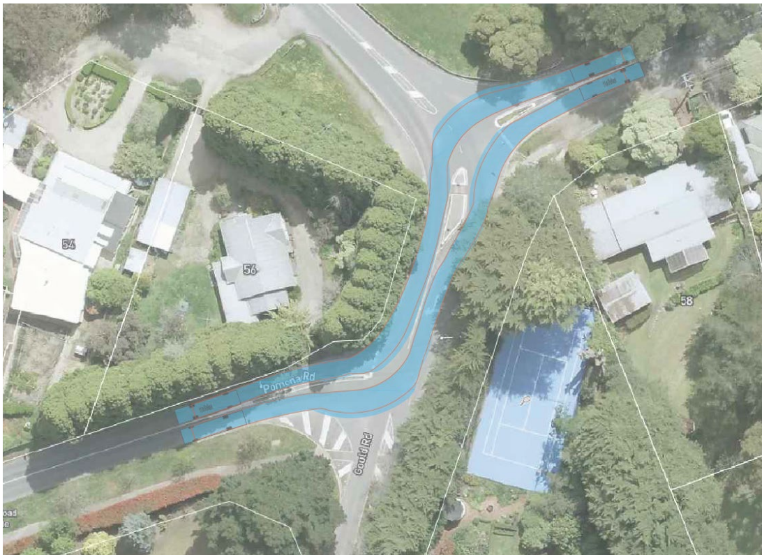
Figure 9 - Indicative commercial vehicle swept paths at the intersections of Gould Road with Old Mount Barker Road and Pomona Road
