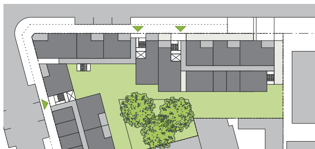
Figure 4F.5 Mixed use buildings may have a range of circulation spaces including multiple cores, gallery access and double-loaded corridors with cross-over apartments
