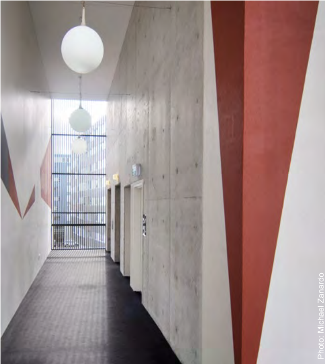
Figure 4F.10 Common circulation spaces should provide short sight lines and be well lit at night
