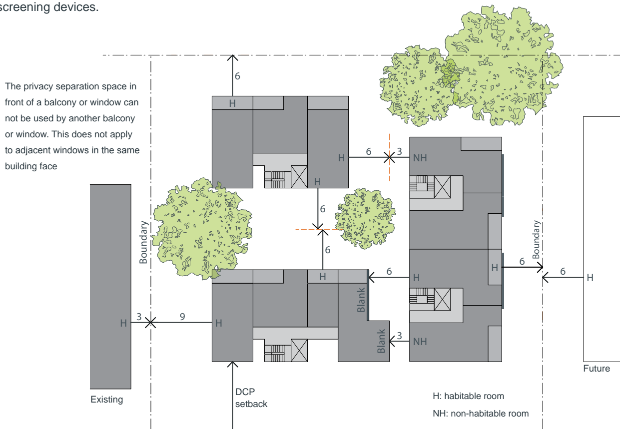
Figure 3F.2 Any one development will have a variety of visual privacy conditions to be accommodated. Section A (Figure 3F.4) shows separation distances between apartments within the same site
