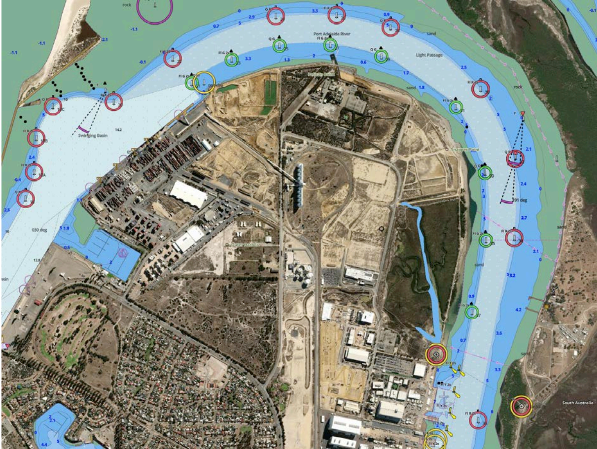
Figure 35: Port River bathymetry (Source: i-Boating nautical map used under licence from Australian Hydrographic Office)
