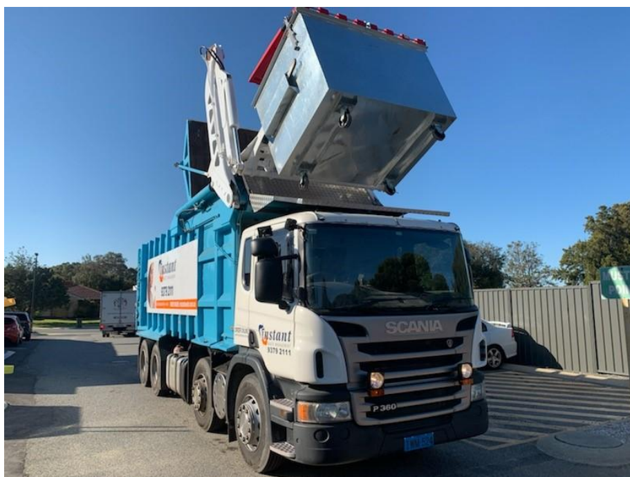
Figure 4-2 – Photo example of a front-lift bin being emptied. Image source: Instant Waste Management
