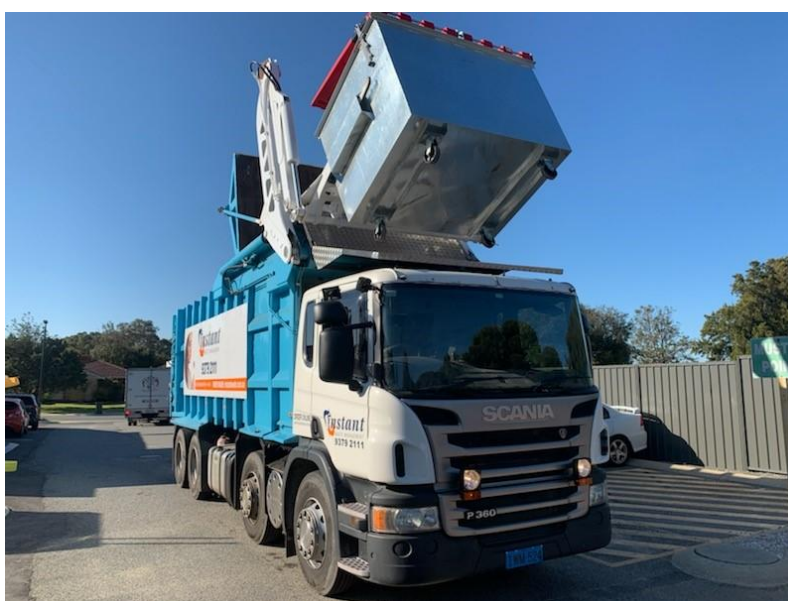
Figure 4-2 – Photo example of a front-lift bin being emptied. Image source: Instant Waste Management
