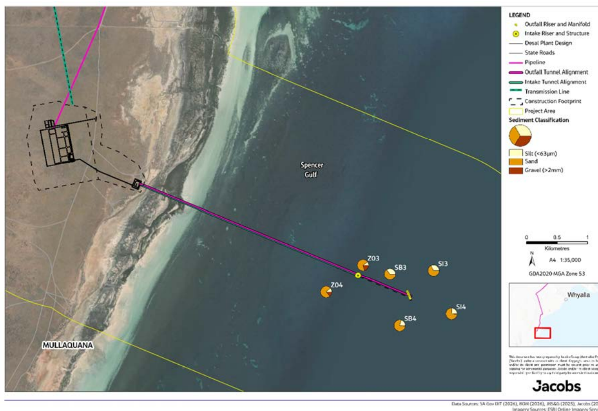
Figure 4-6 Sediment classification: Proportion of silt, sand and gravel per sample location (Data adopted from JBS&G, 2025)
