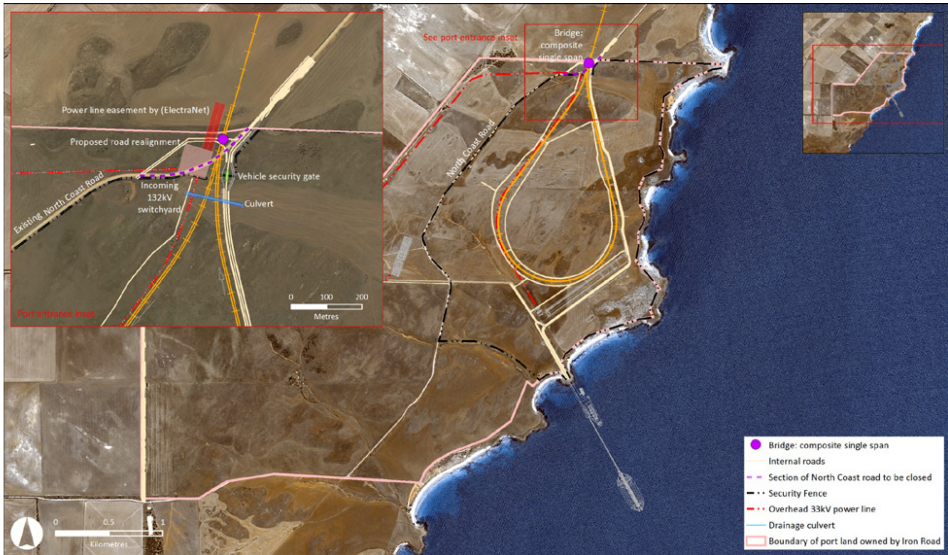
Figure 4-33 Port Site Roads and Access
