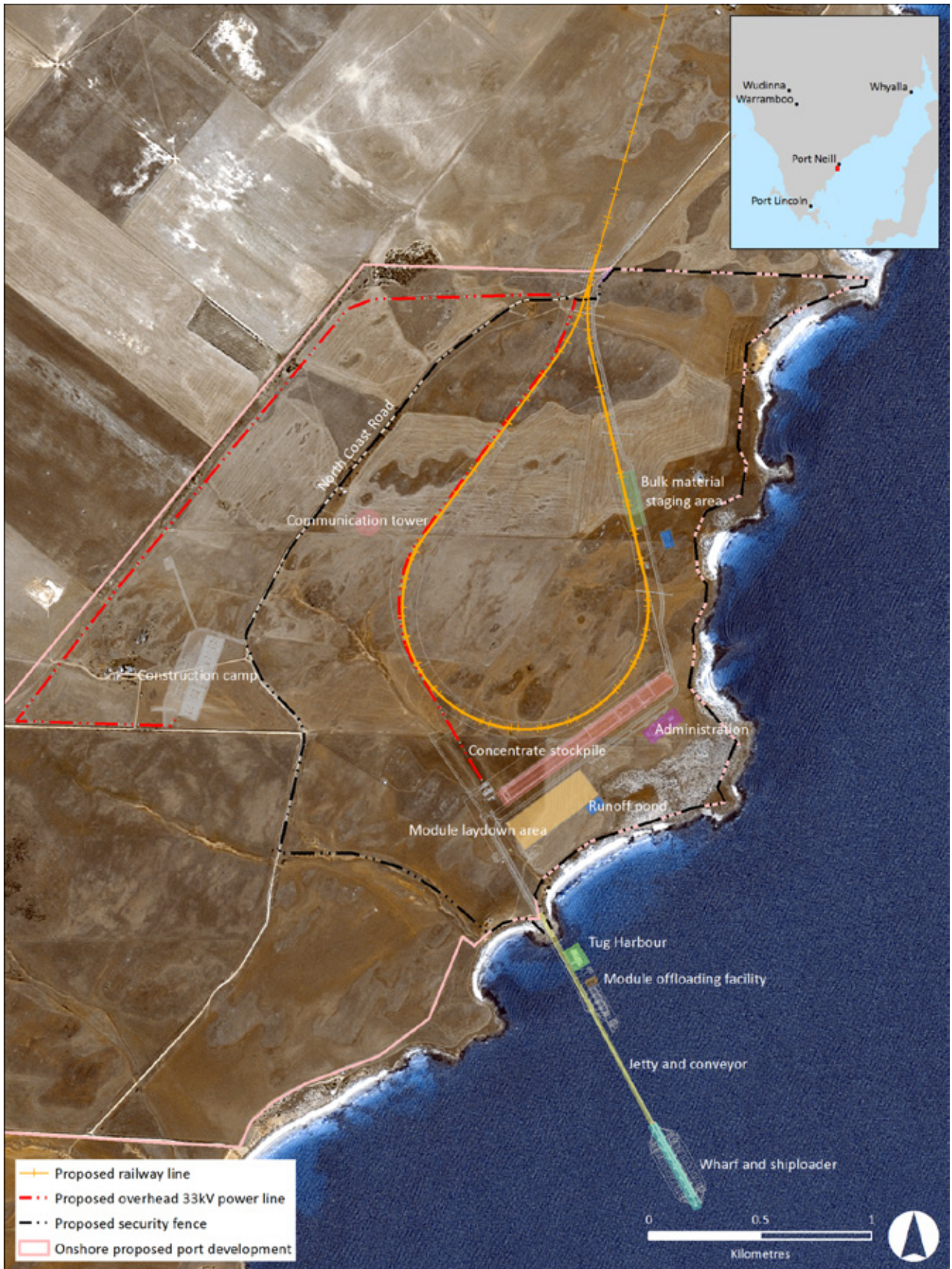
Figure 4-19 Port Site Infrastructure Layout
