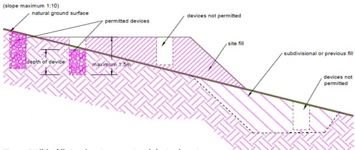
Figure 3.1(b) - fill site showing permitted device location
