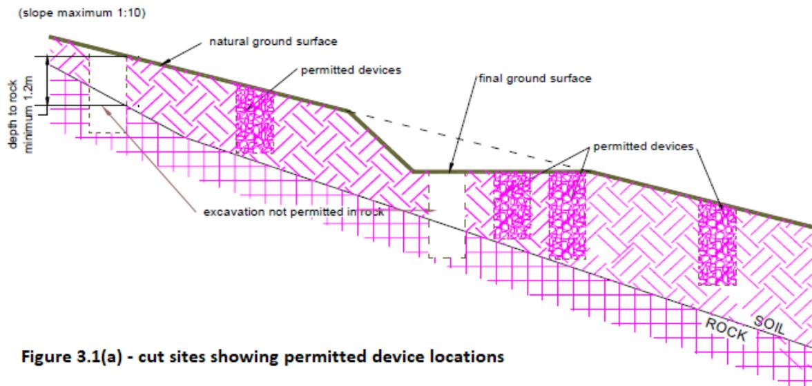
Figure 3.1(a) - cut sites showing permitted device locations
