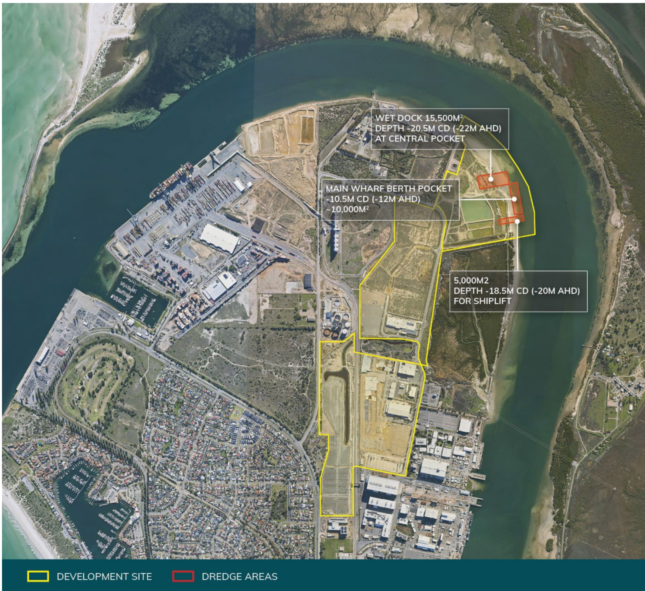
Figure 5.1 - Preliminary dredging areas for the construction of the development
