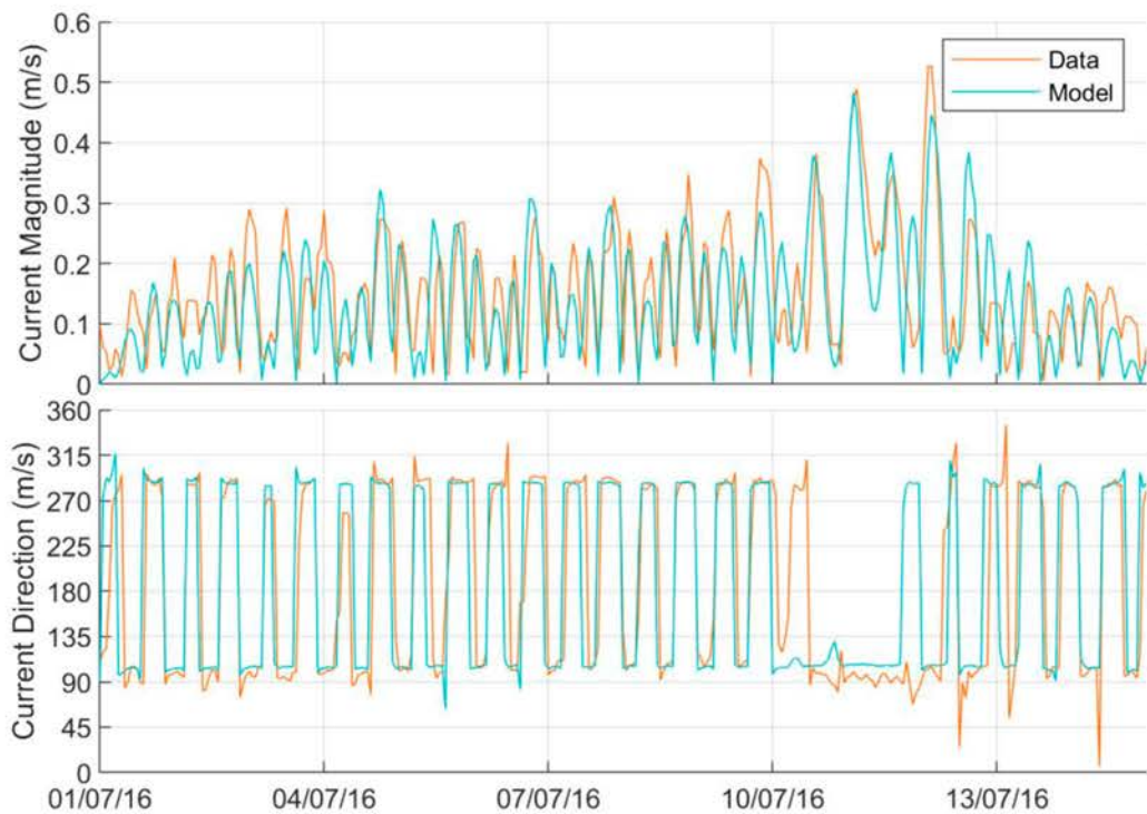
Figure 2-8 Depth-averaged current magnitude and direction timeseries at Wharf Location.
