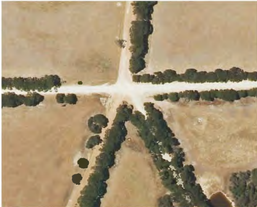
Ropers Road 5 - 5 way intersection that would require reconfiguration and upgrade
