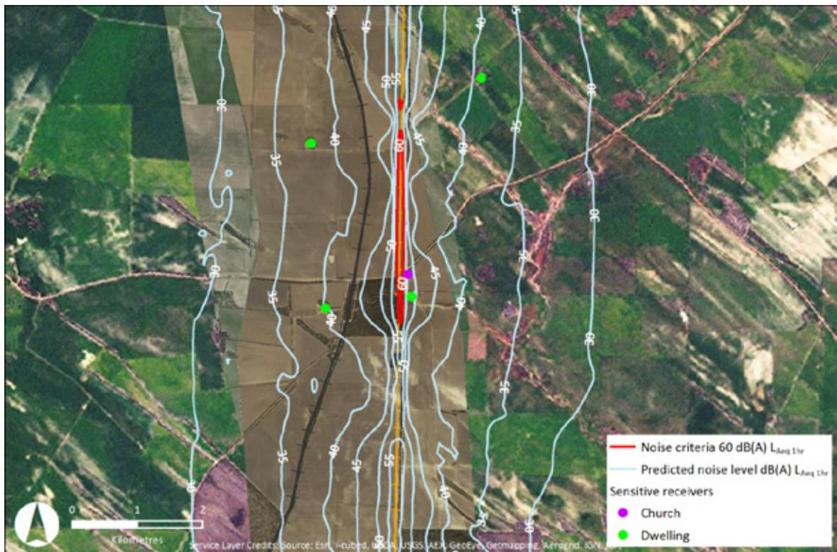
Figure 12-8 Example Enlargement of Predicted Noise Contours, Night  $L_{Aeq 1hr}$  for the Operation of the Railway
