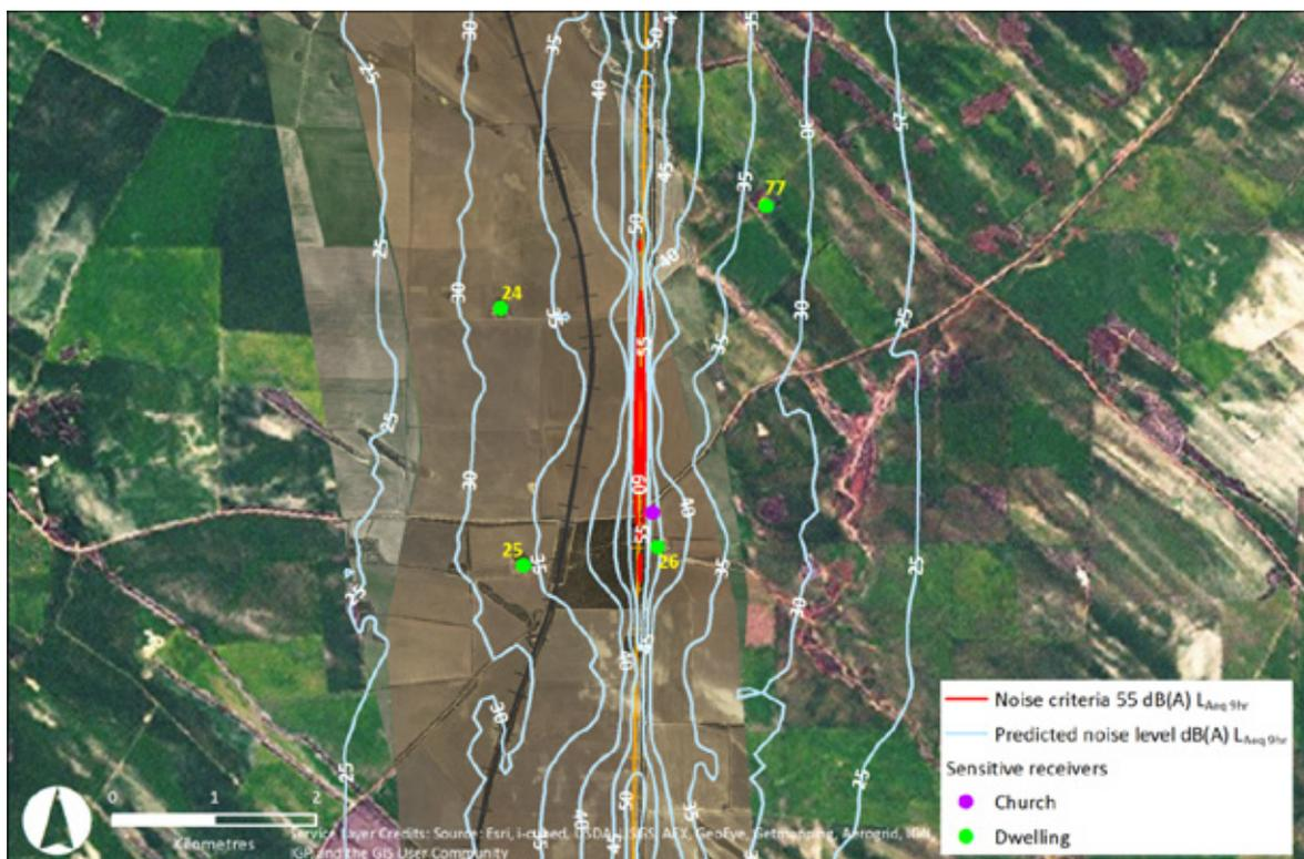
Figure 12-6 Example Enlargement of the Predicted Noise Contours, Night L<sub>Aeq,9hr</sub> for the Operation of the Railway
