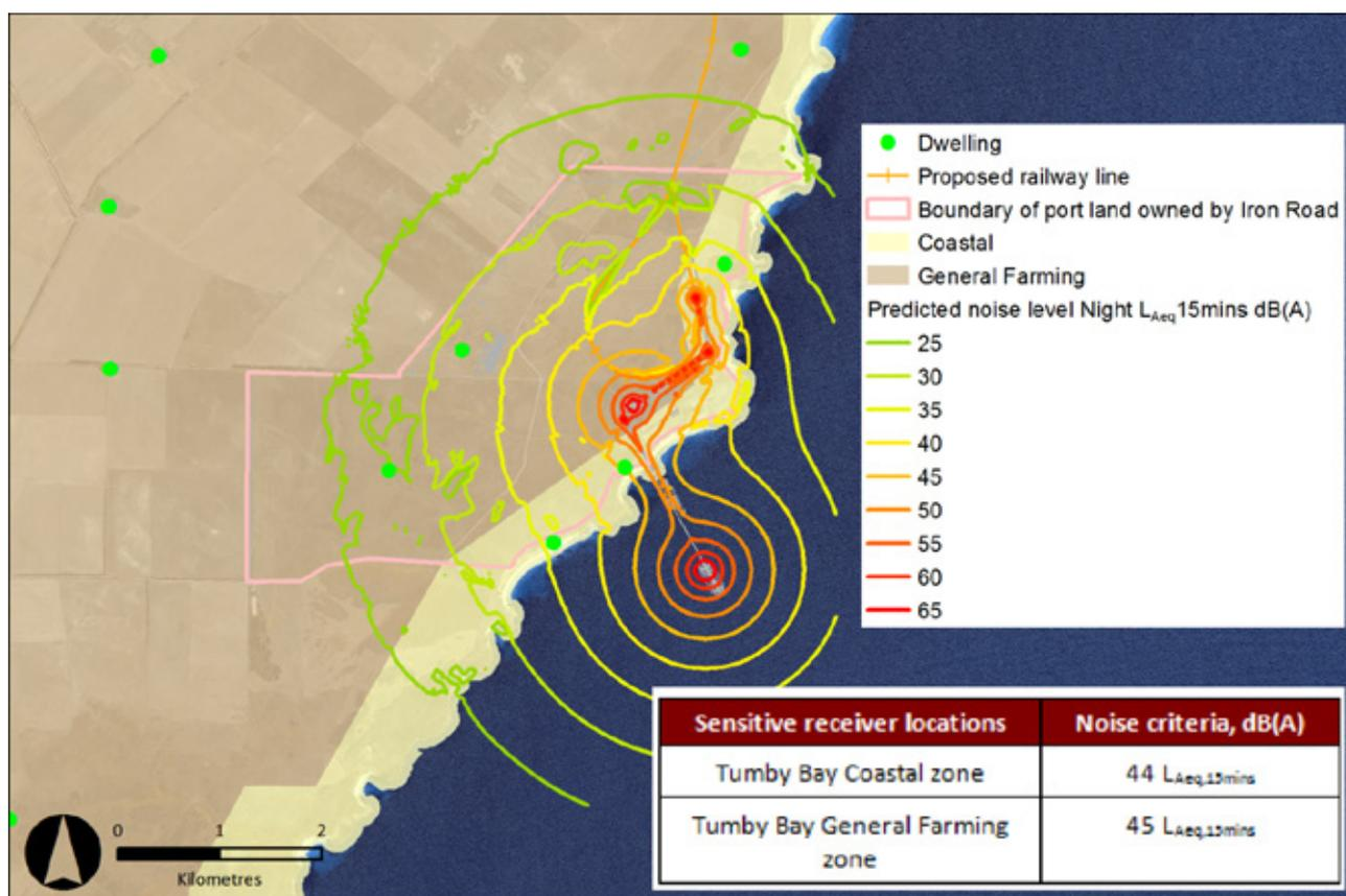
Figure 12-10 Predicted Operational Noise Contours for Proposed Port Development, Night  $L_{Aeq,15mins}$  dB(A)
