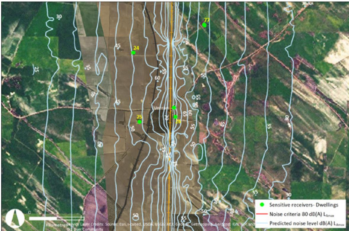
Figure 12-7 Example Enlargement of the Predicted Noise Contours, Night  $L_{Amax}$  for the Operation of the Railway
