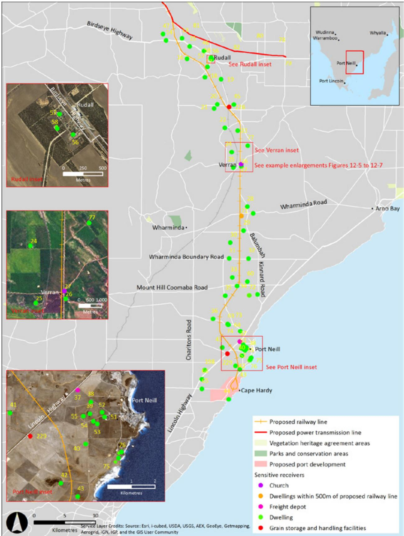
Figure 12-4 Noise and Vibration Sensitive Receivers – Southern Section of Proposed Infrastructure Corridor and Port
