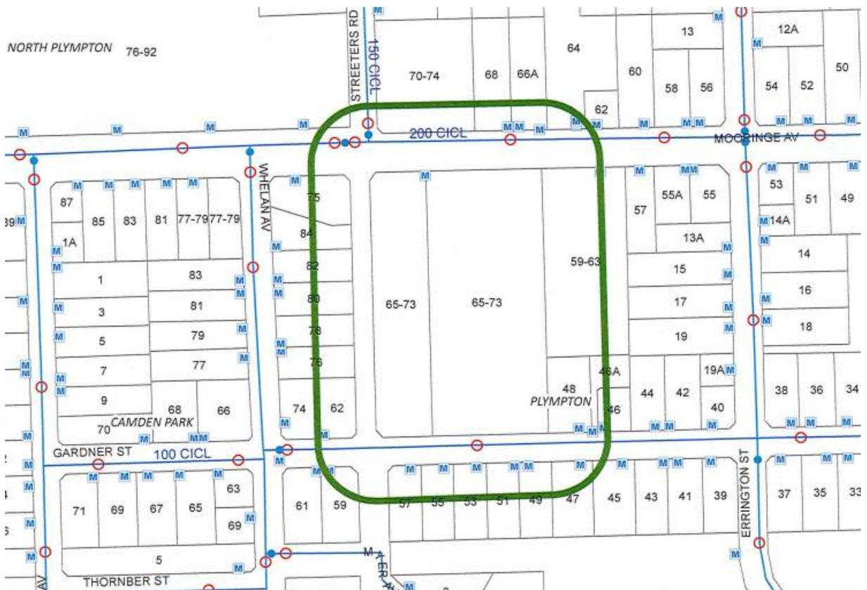
Figure 2 - Potable Water Layout
