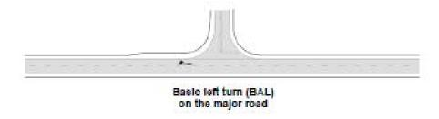
Figure 6-1: Example of a basic left turn (BAL) treatment from major road (Source: Austroads)
