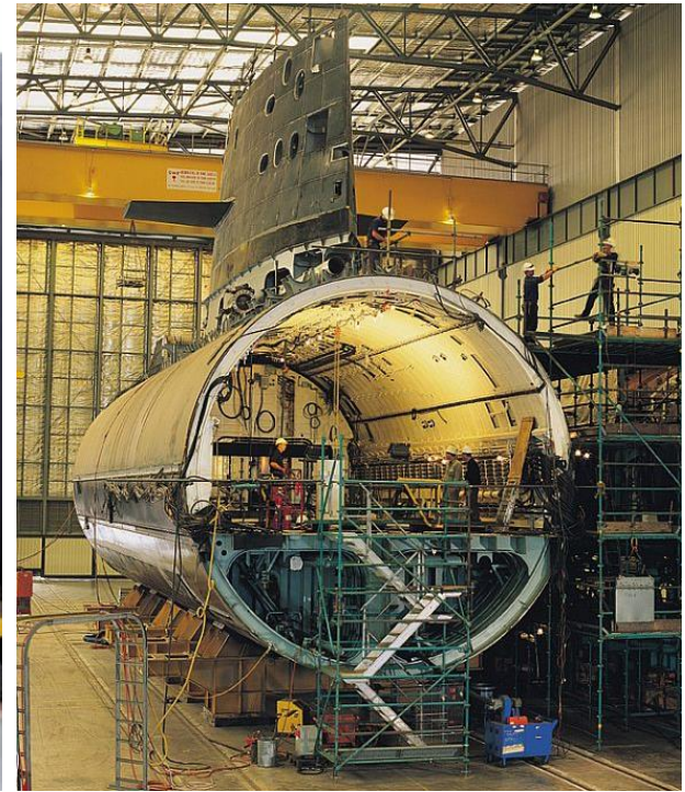
3. Photo of Collins-class submarine under construction in Osborne Naval Shipyard (Source: ADM 2016)
