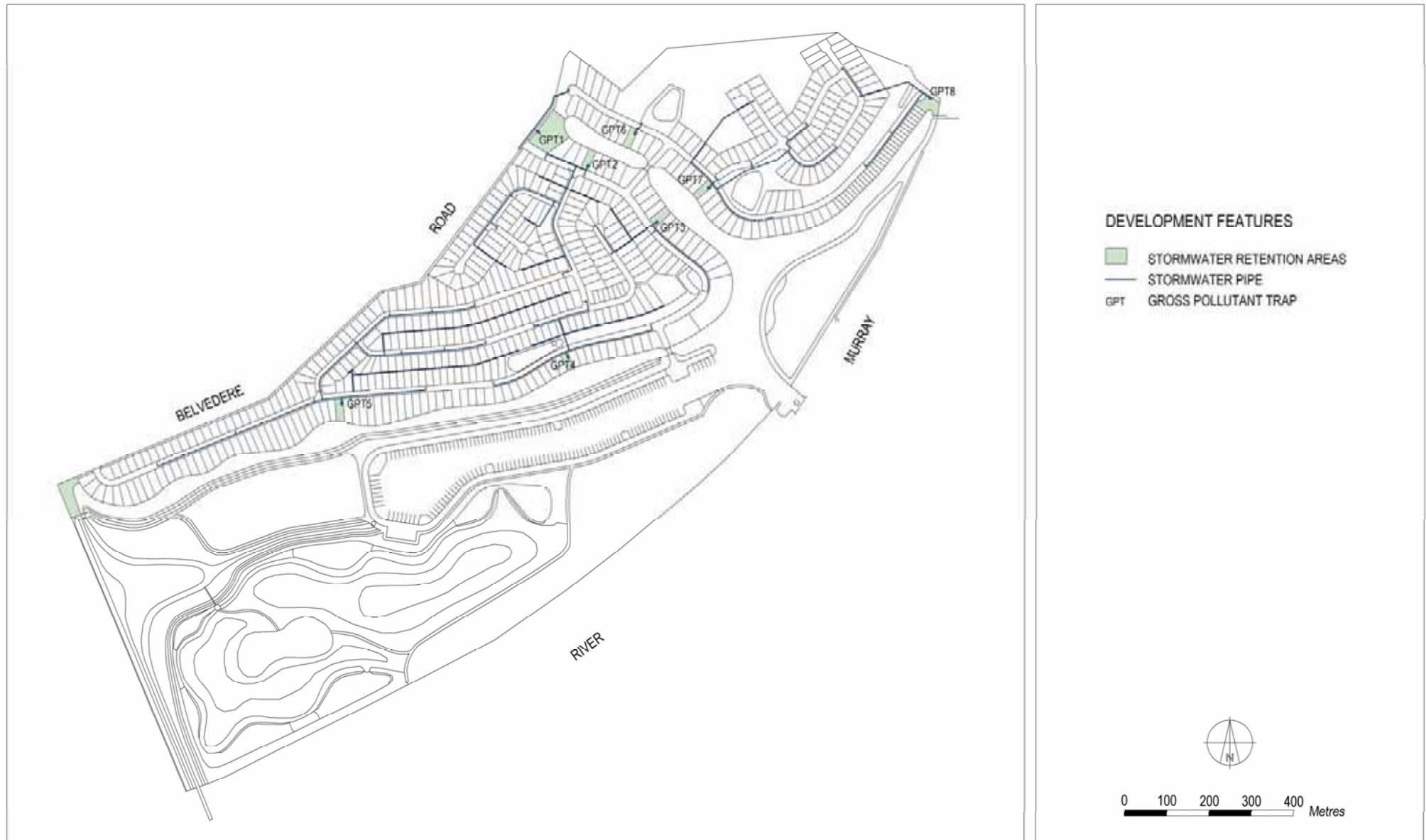
Figure 2.27 – Typical stormwater drainage system
