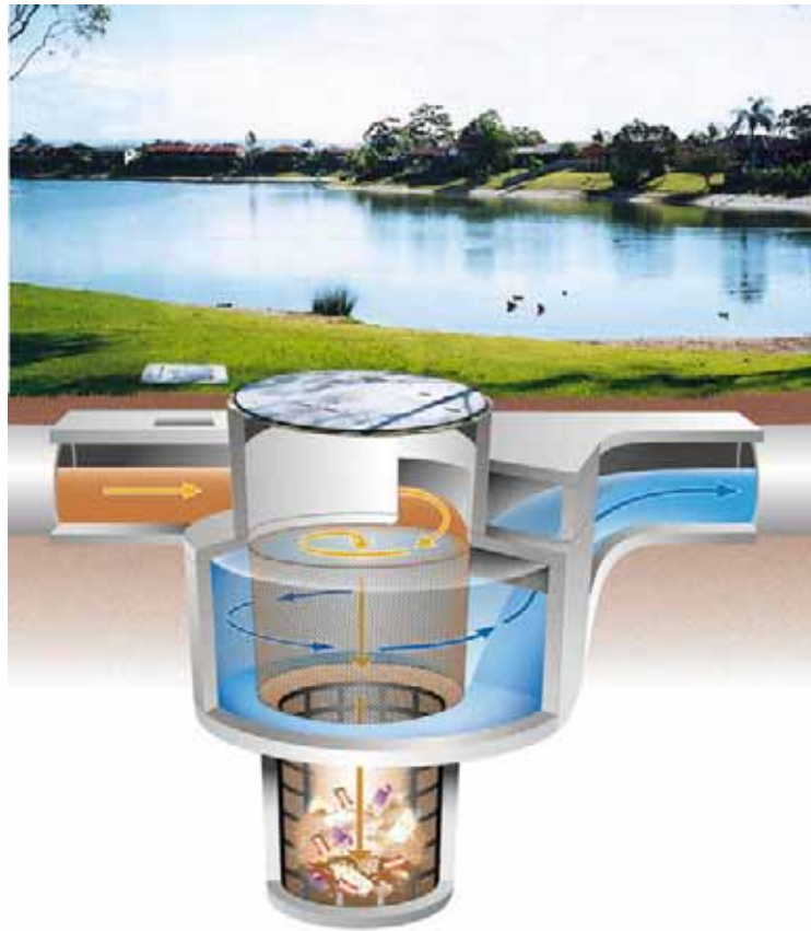
Photo 2.21 – Typical self-cleansing gross pollutant trap
