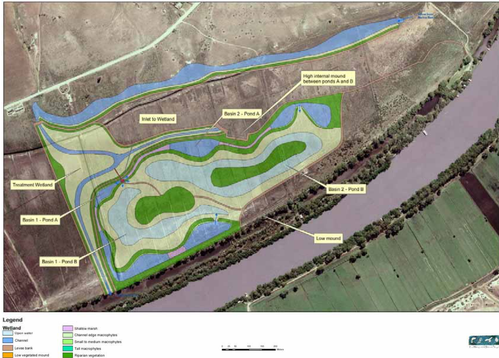
Figure 2.31 – Concept plan for anabranch channel, treatment wetland and ephemeral wetland
