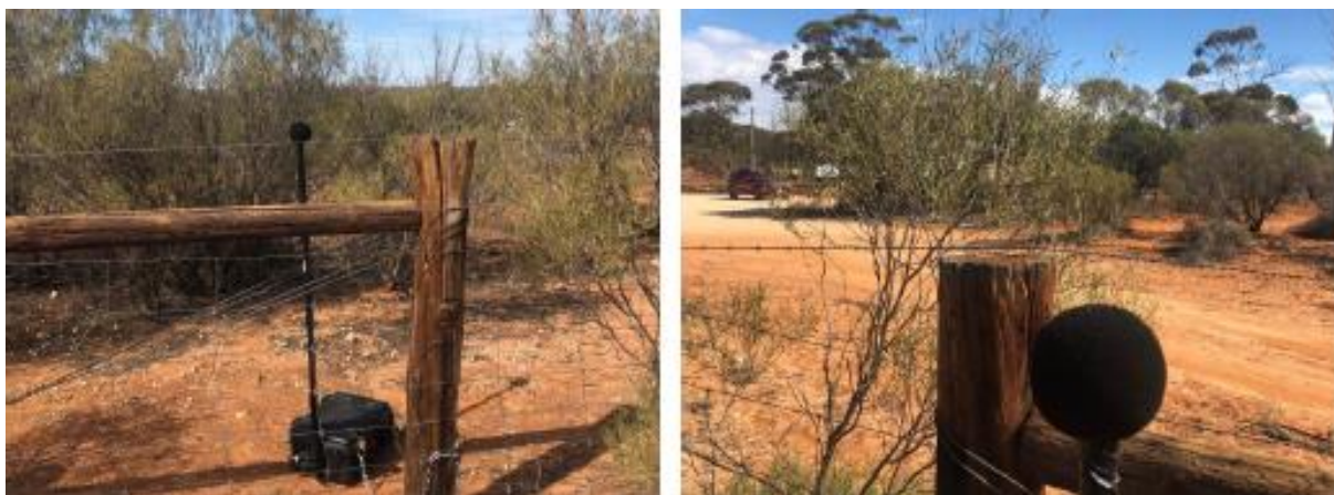
Plate 15-1: Noise logger installation
