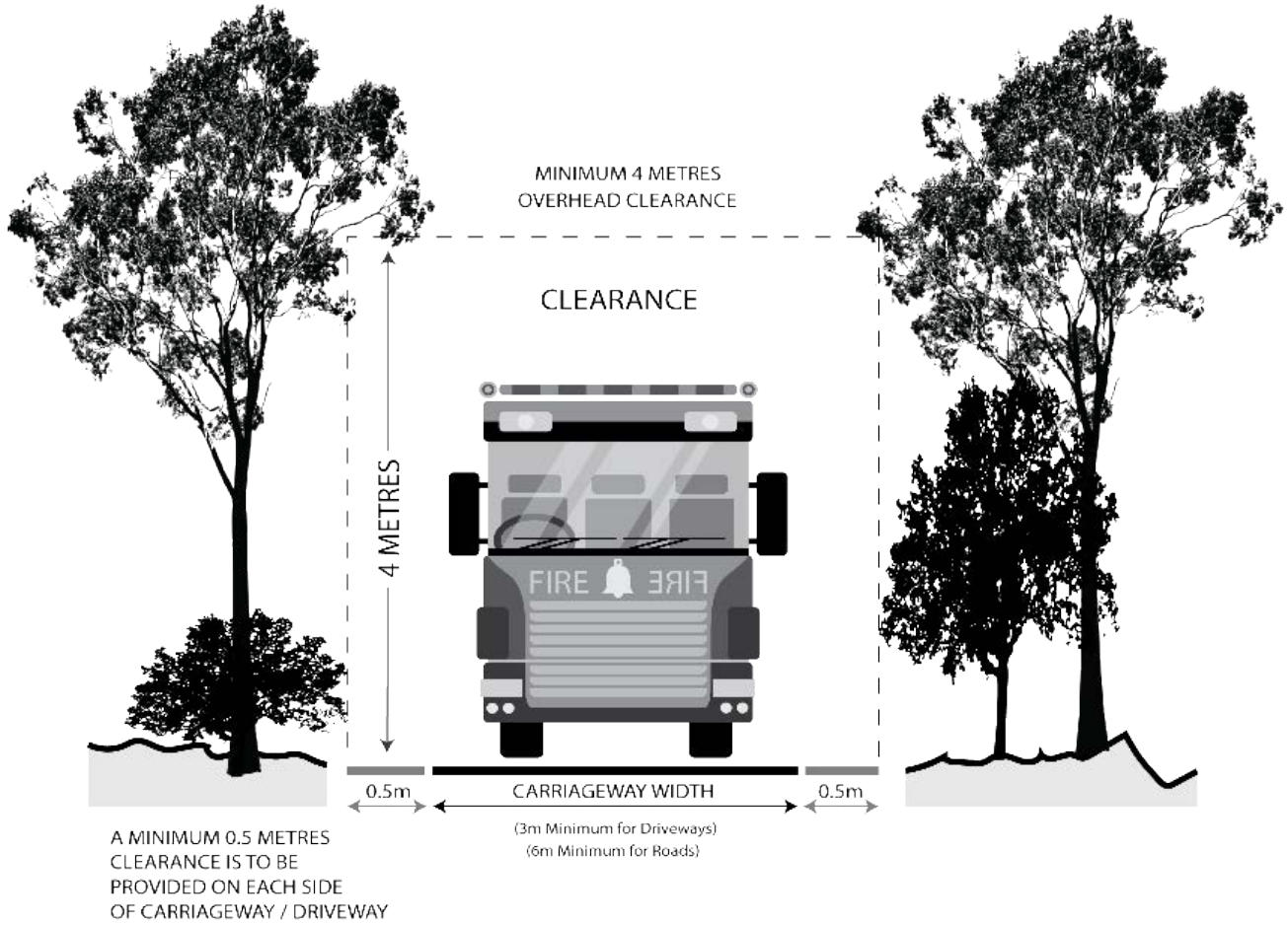
Figure 1 - Overhead and Side Clearances
