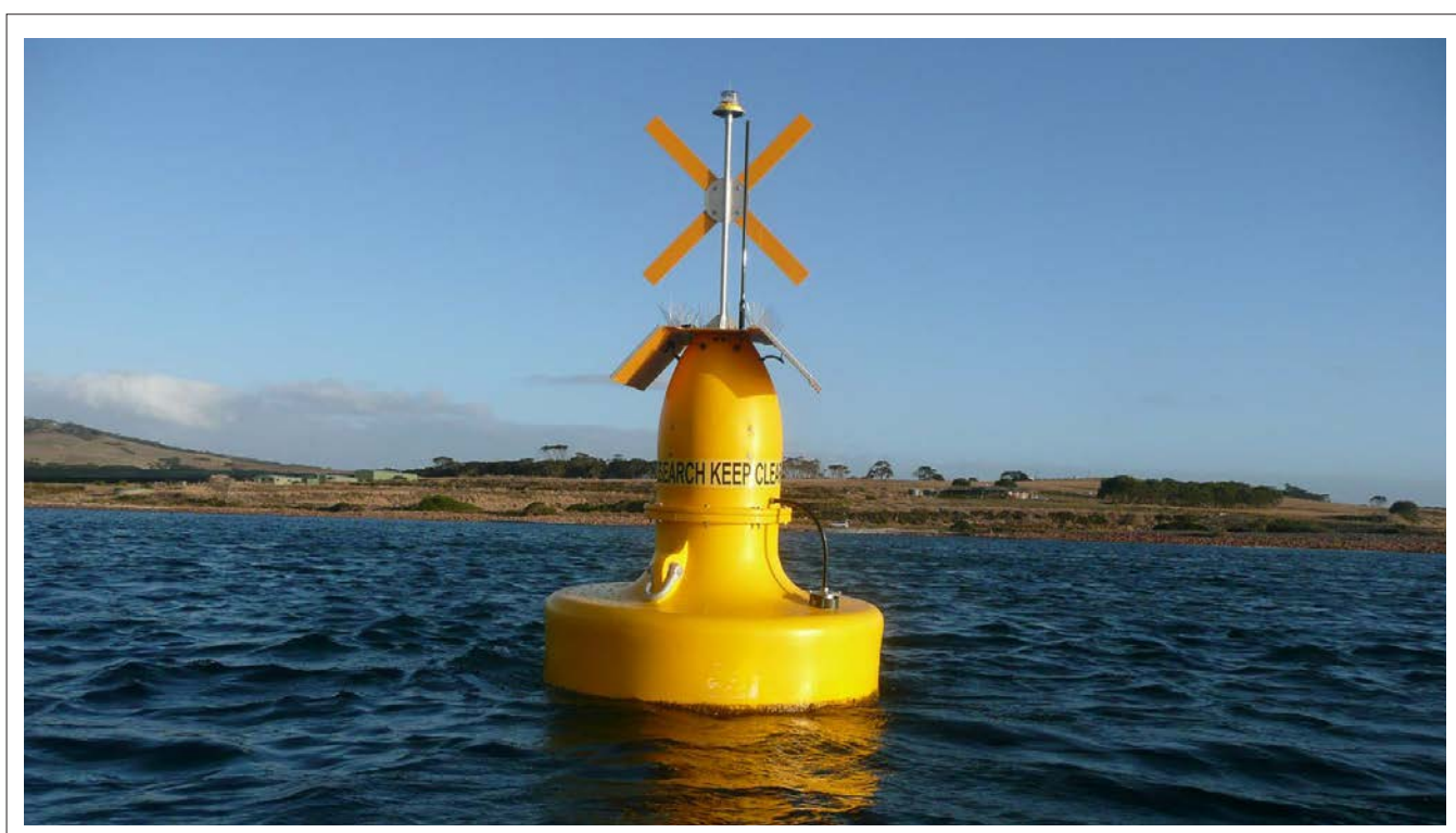
PLATE 9-2 WATER QUALITY MONITORING INSTRUMENT (YSI 6000) DEPLOYED IN SMITH BAY FOR ONE YEAR
