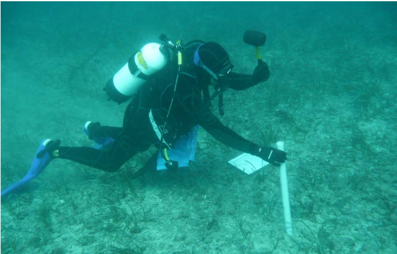
PLATE 9-1 A DIVER TAKING A SEDIMENT CORE IN SMITH BAY (DEPTH 13 M)
