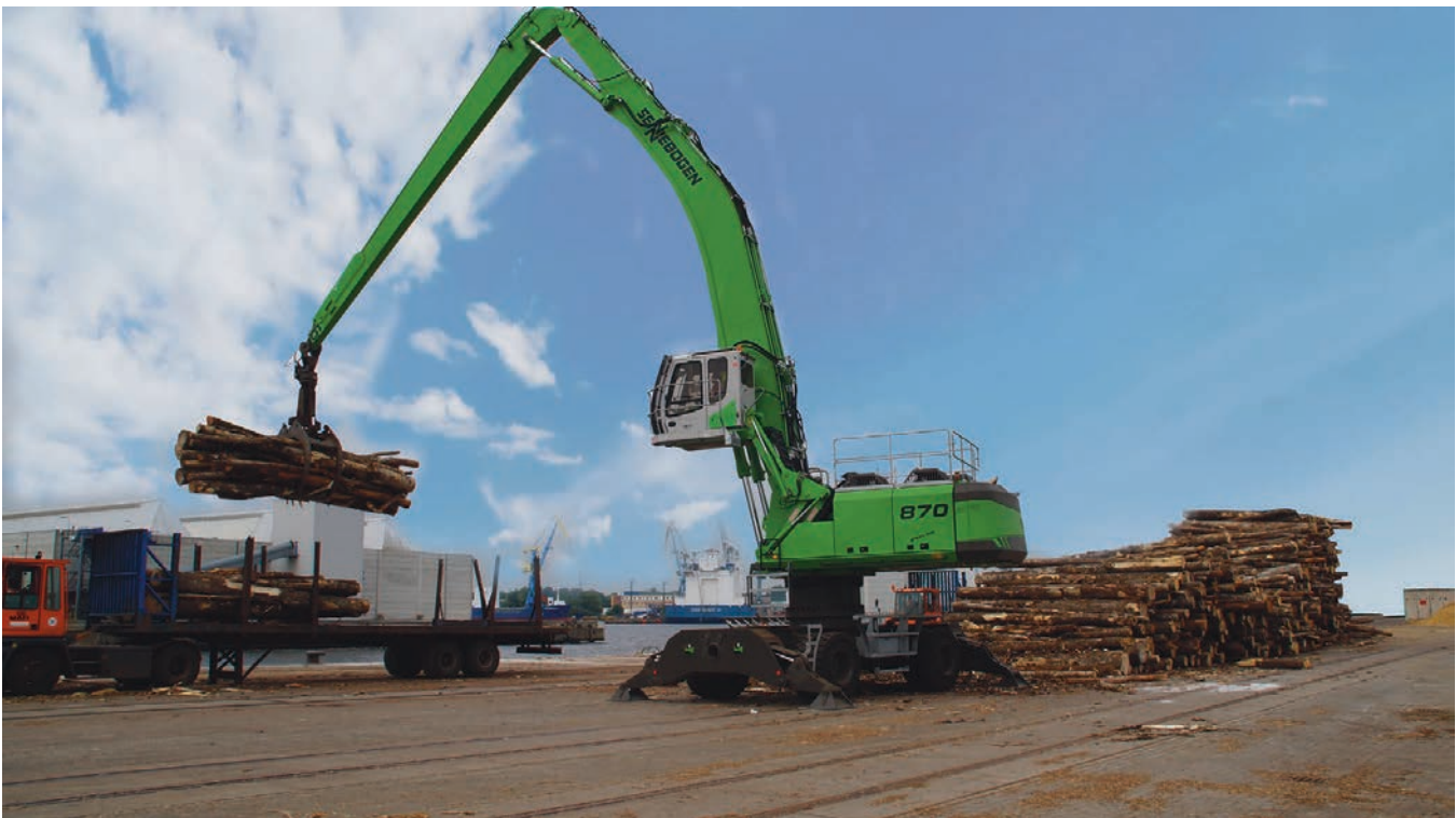
PLATE 4-1 TYPICAL LOG HANDLING MOBILE EQUIPMENT
