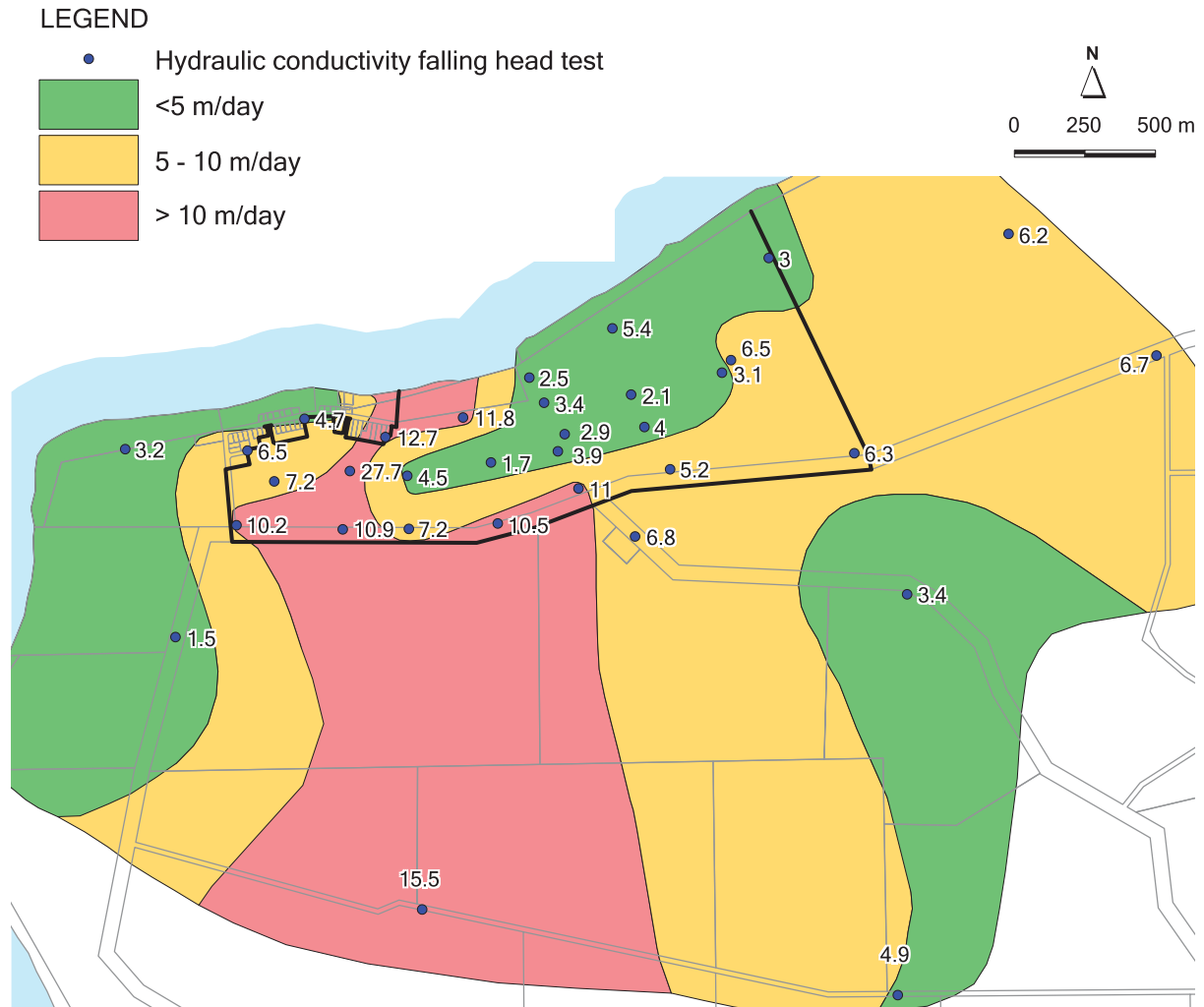
Figure 4.76: Unconfined Aquifer Hydraulic Conductivity - Measured by Falling Head
