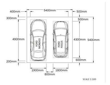
The dimensions for garages used in the Code are based on Australia Standard AS/NZS 2890.1:2004, which uses vehicles sales data from 2000.
