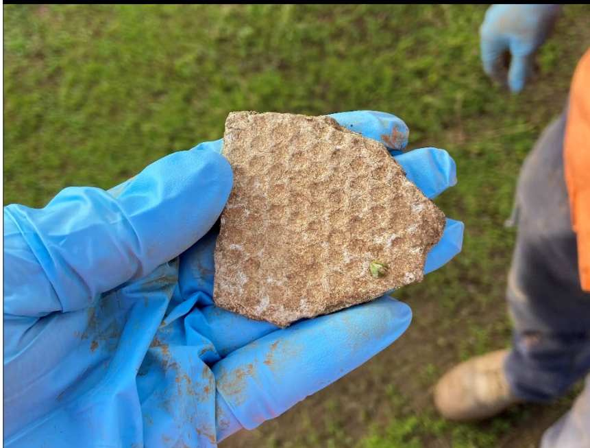
PHOTOGRAPH 12 – VIEW OF ASBESTOS CONTAINING MATERIAL AT SURFACE
