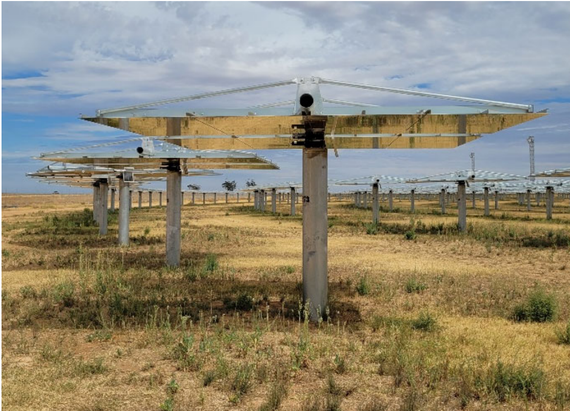
Figure 14: Heliostat in park position (non-operational) with mirrors facing the ground at RayGen's Carwarp demonstration facility.
