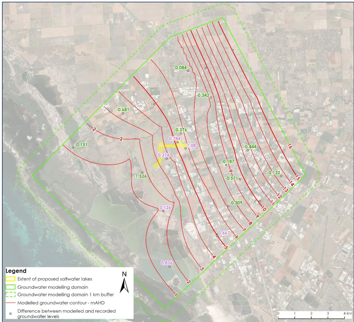
Figure A12. Differences between modelled and recorded groundwater levels
