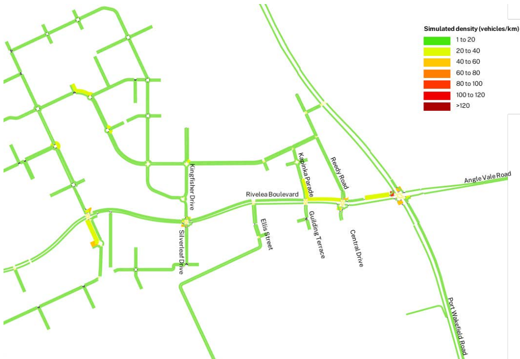
Figure 21: Stage 2 morning peak hour modelled density
