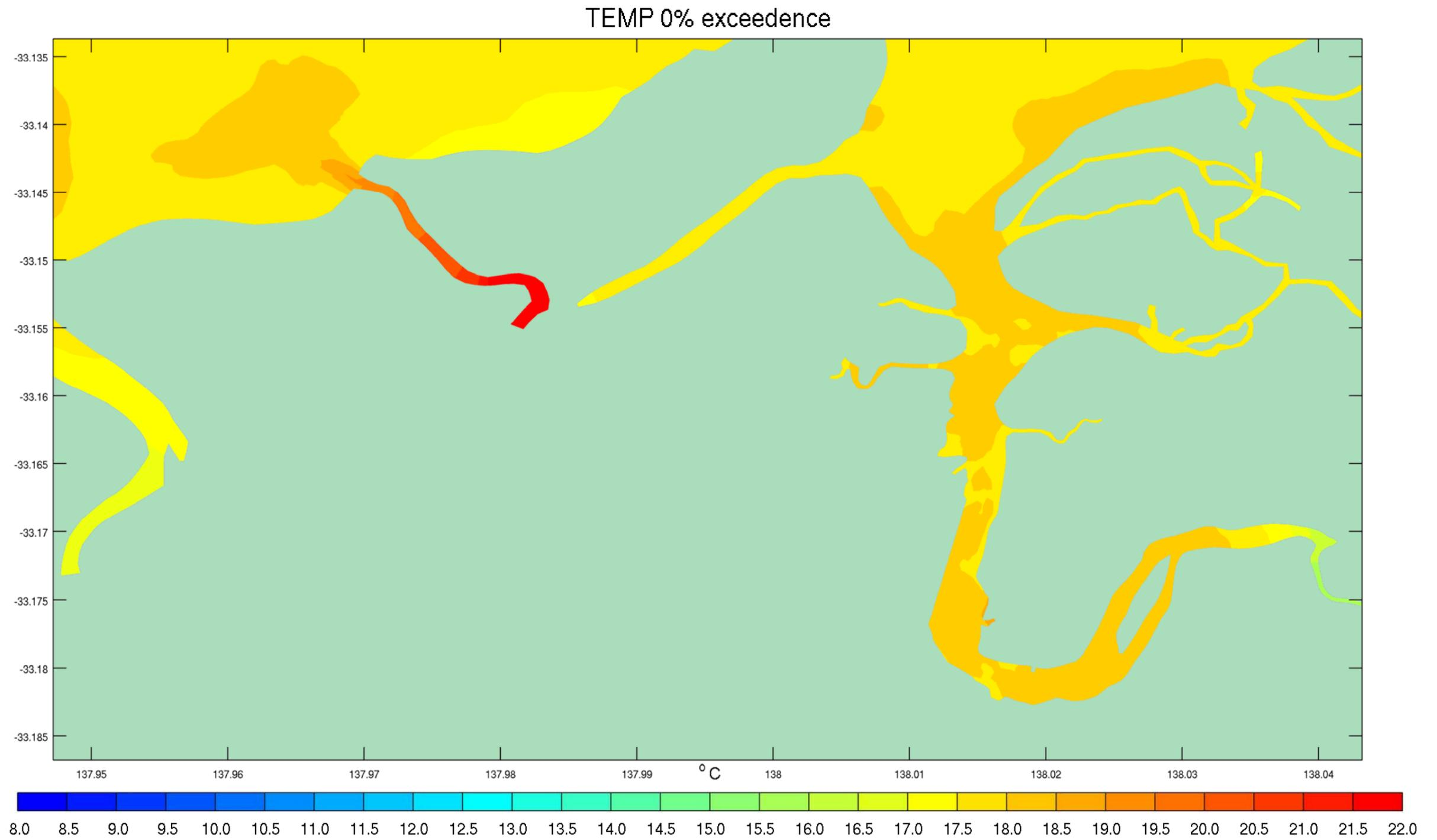
Figure D- 7 0<sup>th</sup> Percentile Temperature Exceedences – Discharge Scenario Conditions September 2012
