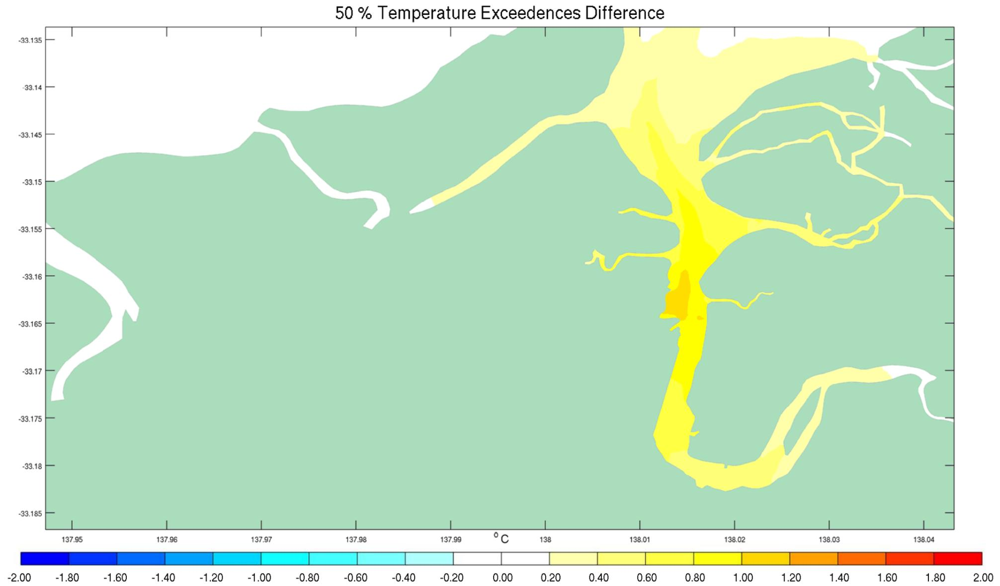
Figure F-12 50<sup>th</sup> Percentile Temperature Exceedences Difference between Discharge Scenario and Existing Conditions July to September 2012
