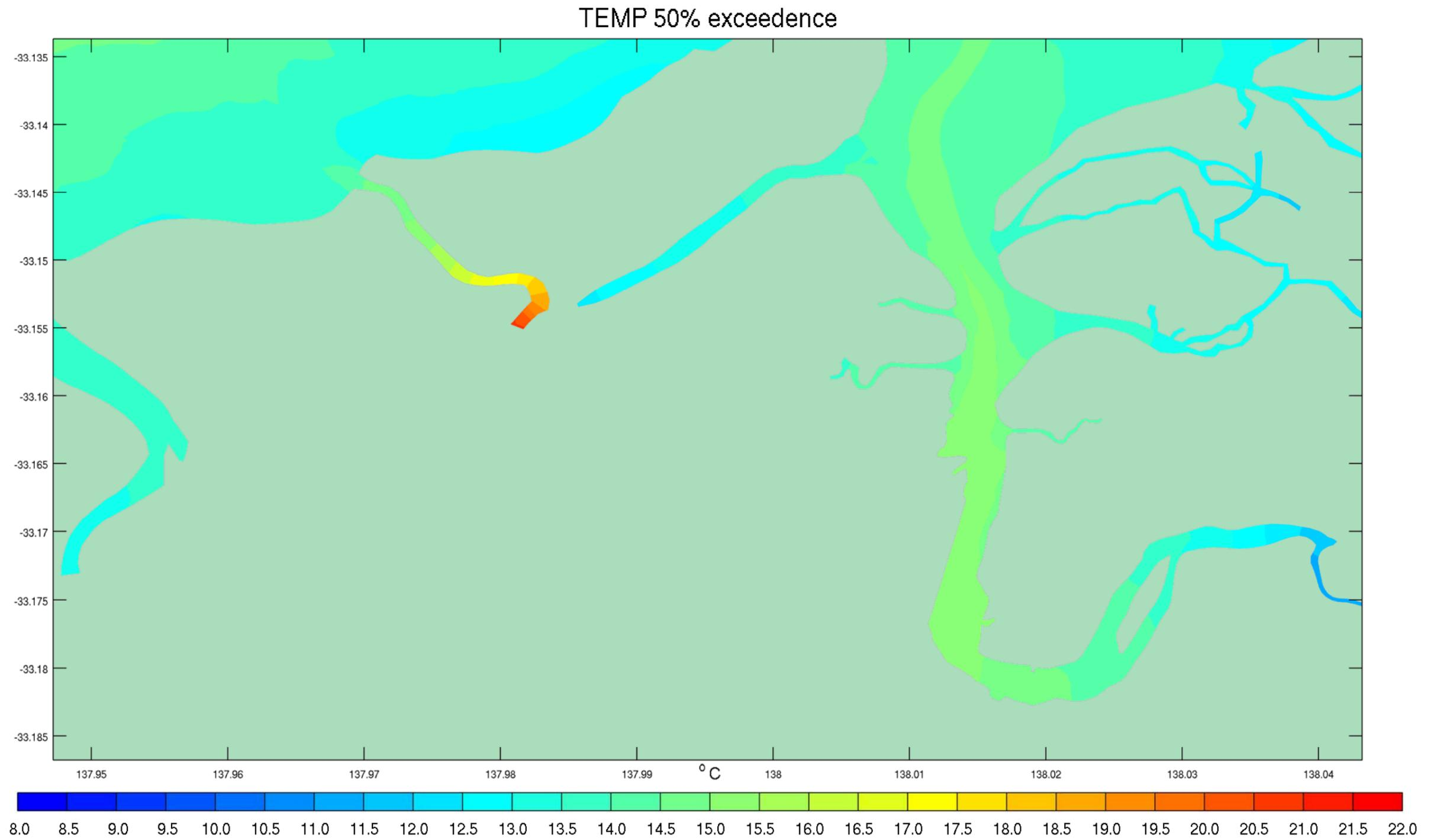
Figure D- 9 50<sup>th</sup> Percentile Temperature Exceedences – Discharge Scenario Conditions September 2012
