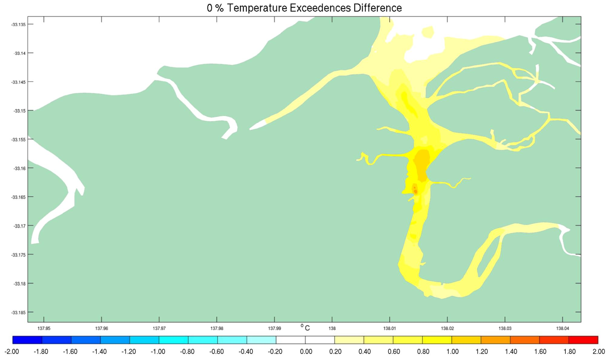
Figure F-10 0<sup>th</sup> Percentile Temperature Exceedences Difference between Discharge Scenario and Existing Conditions July to September 2012
