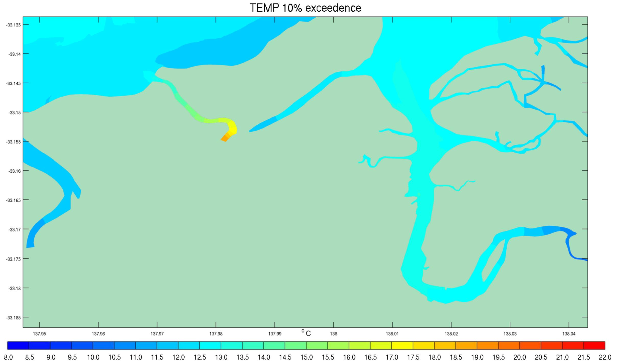
Figure D- 5 10<sup>th</sup> Percentile Temperature Exceedences – Discharge Scenario Conditions August 2012
