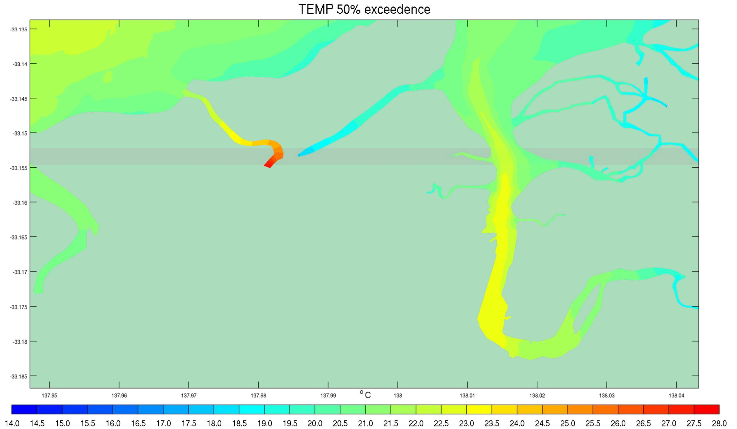
Figure C-9 50<sup>th</sup> Percentile Temperature Exceedences – Discharge Scenario Conditions March 2013
