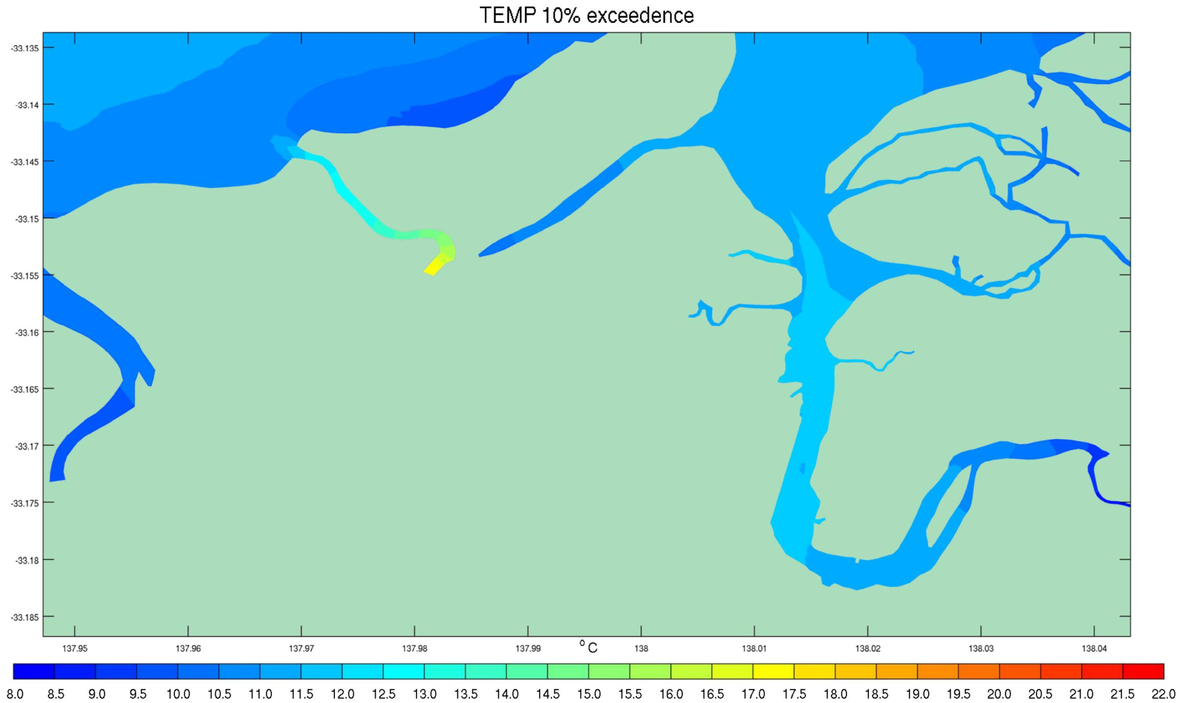
Figure 4-20 10<sup>th</sup> Percentile Temperature Exceedences – Discharge Scenario Conditions July 2012
