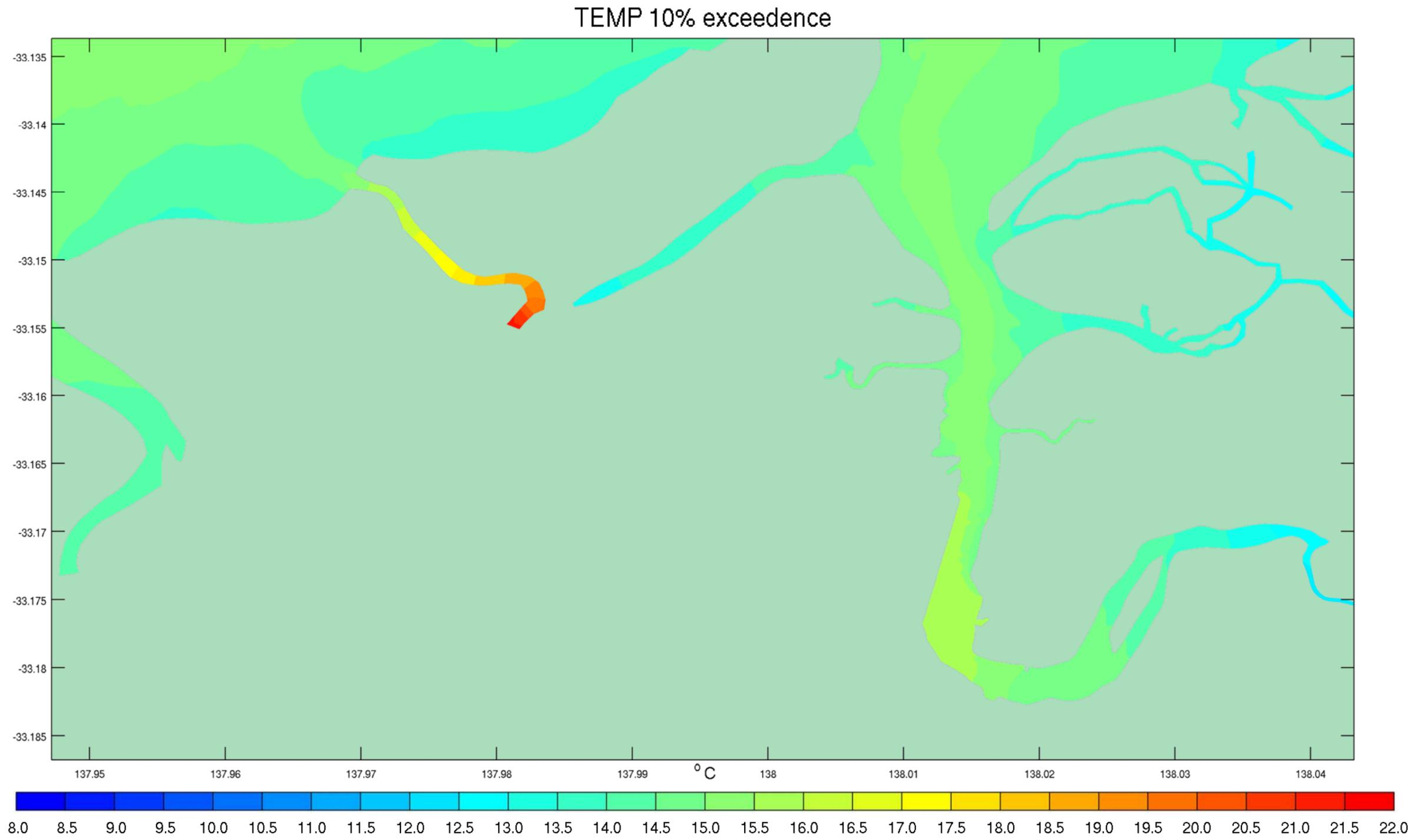
Figure 4-15 10<sup>th</sup> Percentile Temperature Exceedences – Existing Conditions July to September 2012
