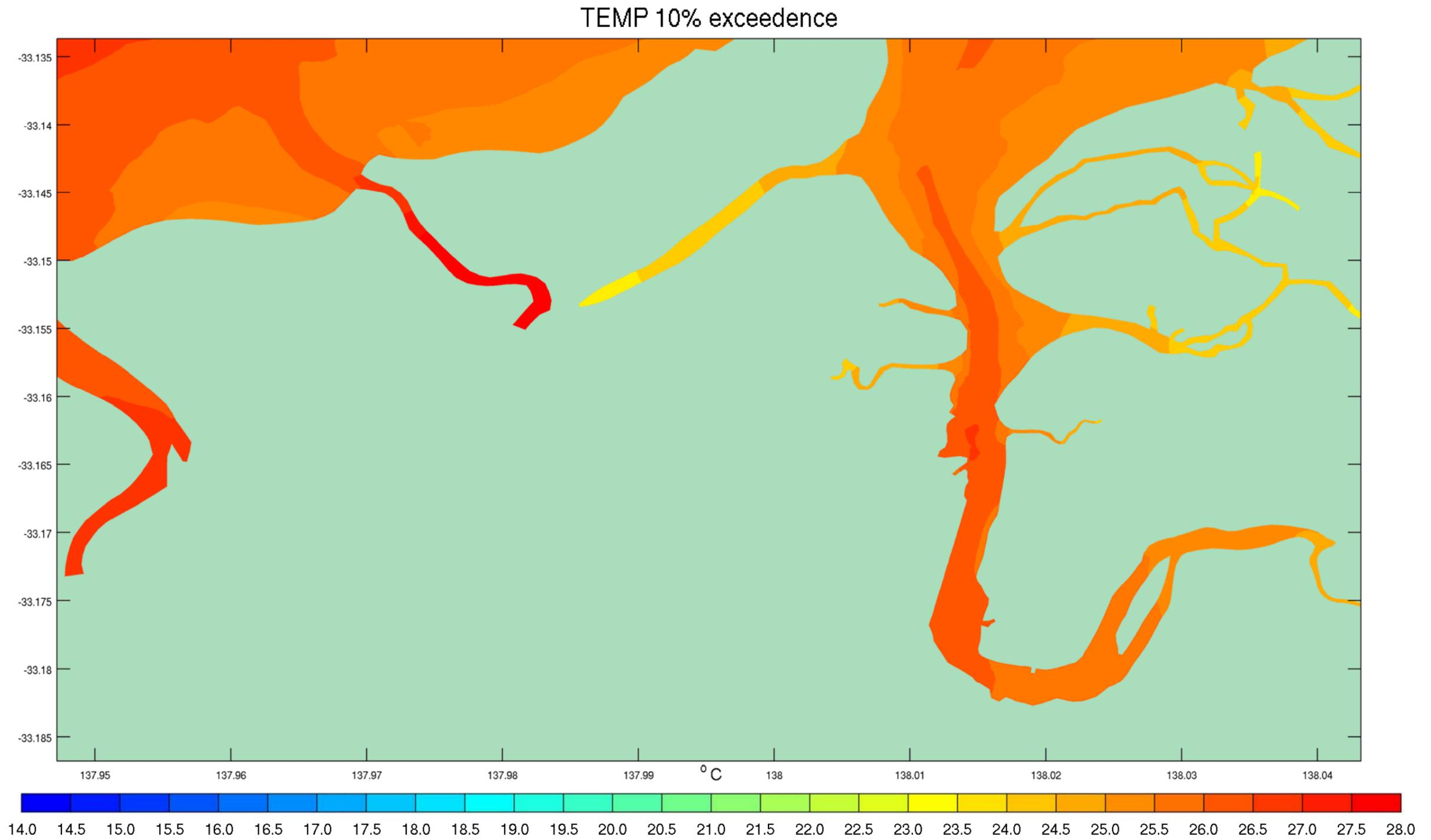
Figure 4-18 10<sup>th</sup> Percentile Temperature Exceedences – Discharge Scenario Conditions March 2013
