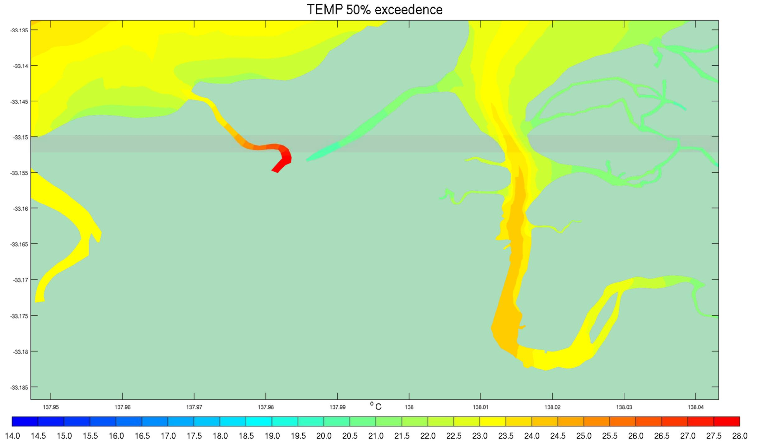
Figure C-6 50<sup>th</sup> Percentile Temperature Exceedences – Discharge Scenario Conditions February 2013
