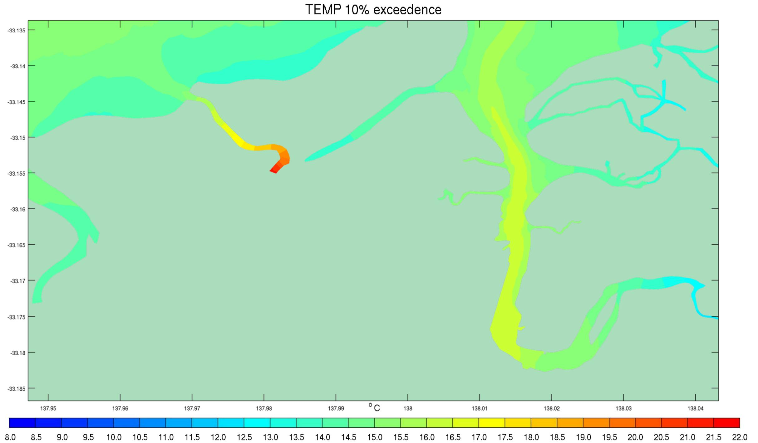
Figure D- 11 10<sup>th</sup> Percentile Temperature Exceedences – Discharge Scenario Conditions July to September 2012
