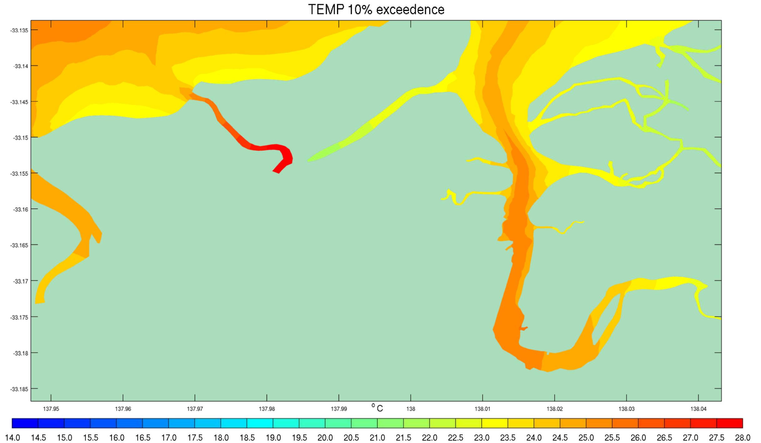
Figure C-2 10<sup>th</sup> Percentile Temperature Exceedences – Discharge Scenario Conditions January 2013
