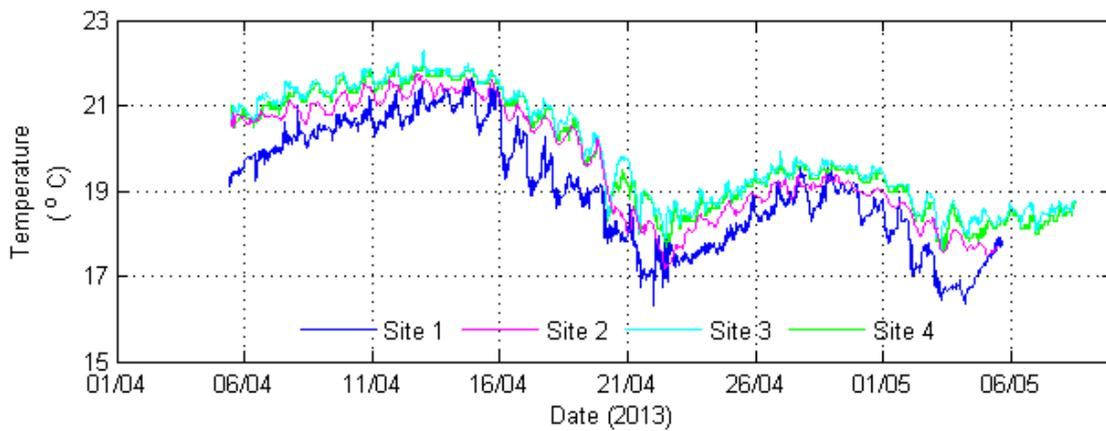
**Figure 2-5 CTD Temperature Measurements – Comparisons at Surface between All Sites**
