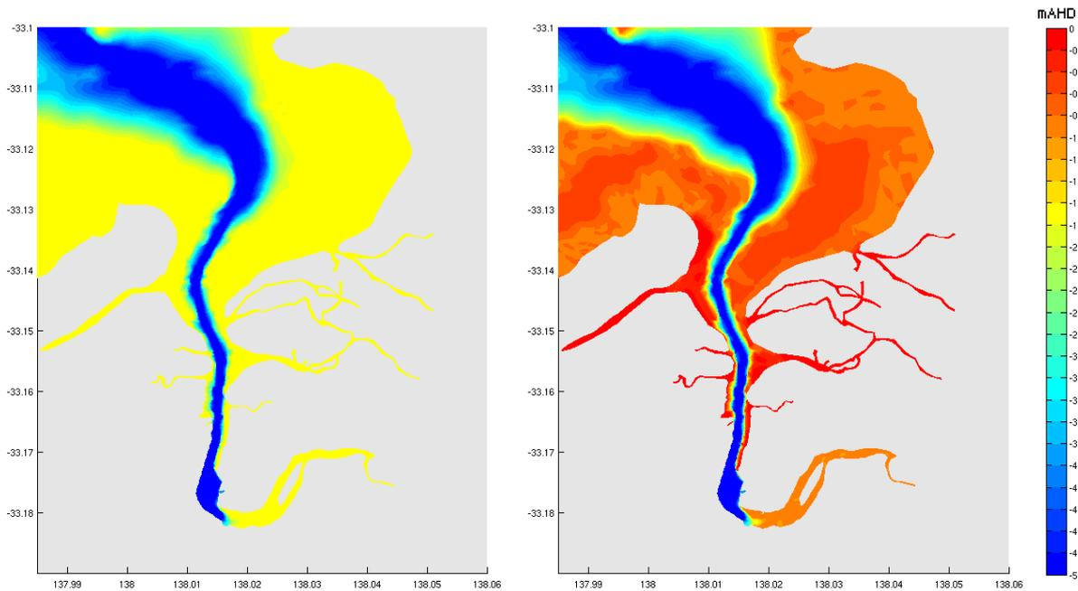
**Figure 4-4 Development of Bathymetry in the Intertidal Areas near Port Pirie. Left Panel: Intertidal areas at a constant elevation corresponding to 0.0 m LAT (~ -1.7 m AHD). Right Panel: Arbitrarily adjusted bathymetry.**
