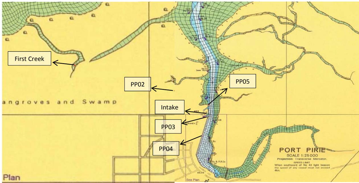
**Figure 4-2 Numerical Mesh near Port Pirie. The mesh is superimposed on AUS 136 charts (AHS 2000). The images are a composite of the Approaches to Whyalla chart and the Port Pirie chart. Scale shown does not apply.**
