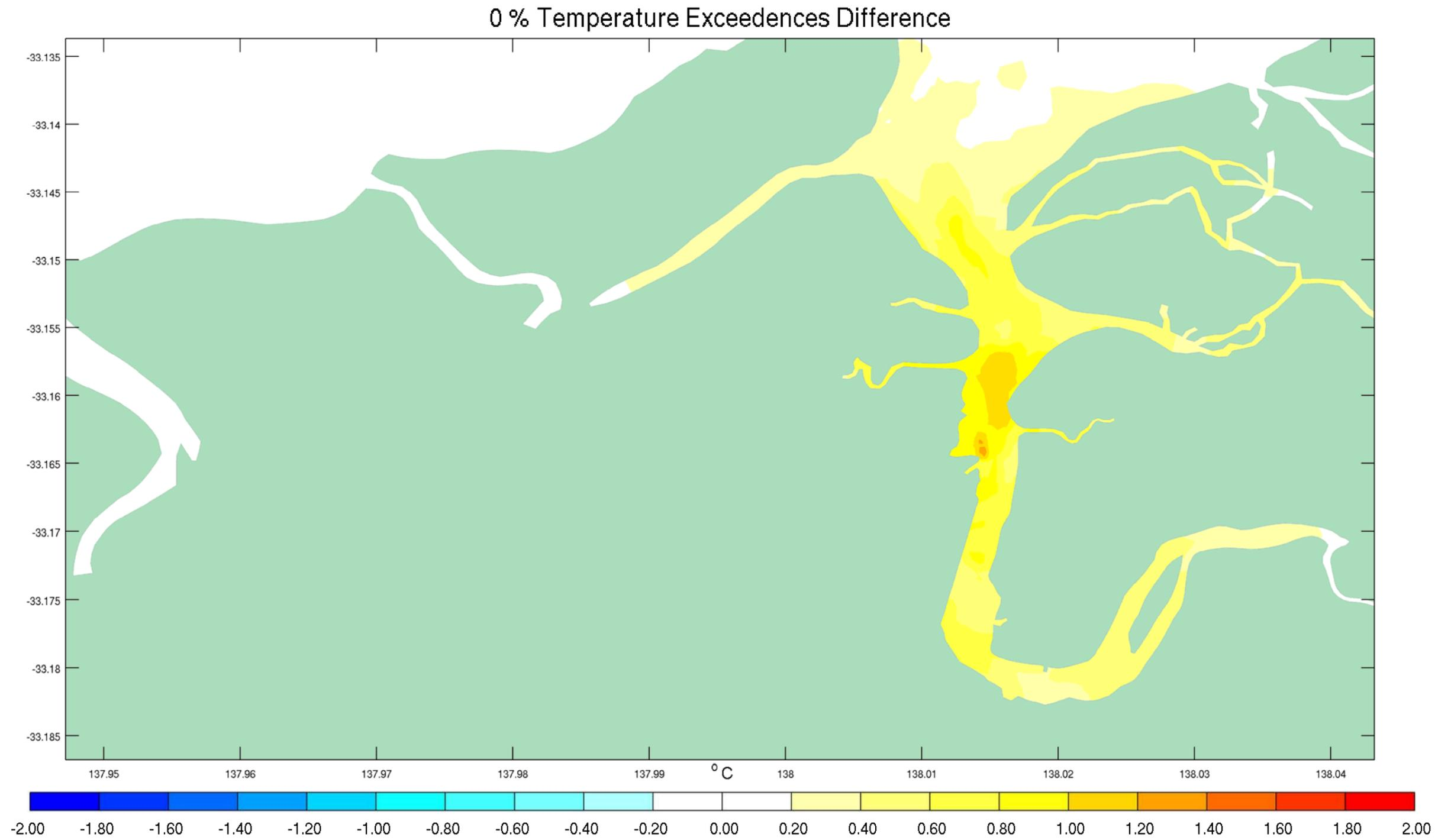
Figure F-7 0<sup>th</sup> Percentile Temperature Exceedences Difference between Discharge Scenario and Existing Conditions September 2012
