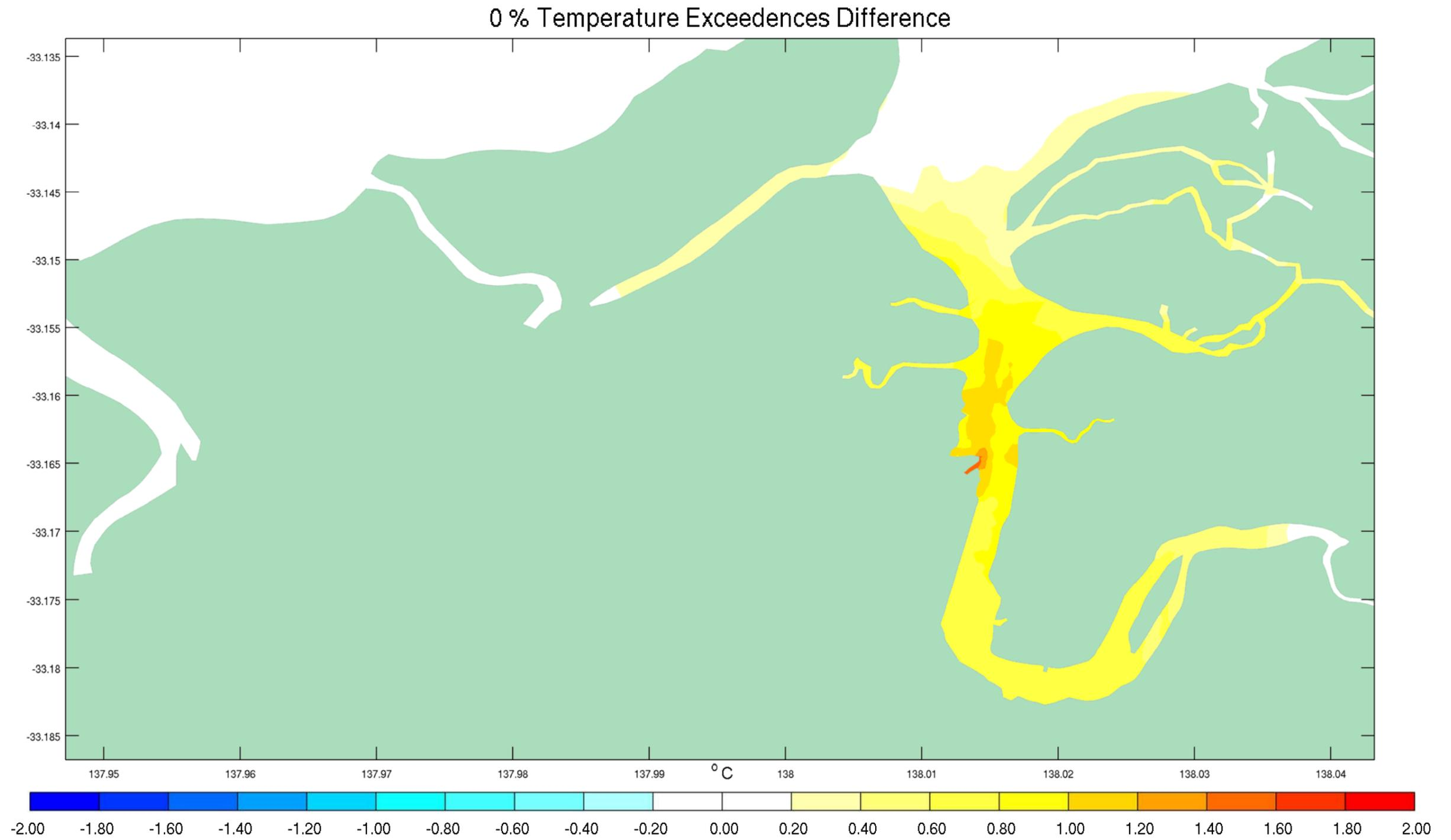
Figure E-7 0<sup>th</sup> Percentile Temperature Exceedences Difference between Discharge Scenario and Existing Conditions March 2013
