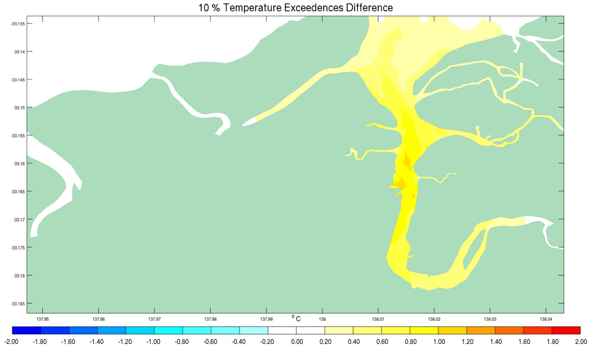
Figure F-11 10<sup>th</sup> Percentile Temperature Exceedences Difference between Discharge Scenario and Existing Conditions July to September 2012
