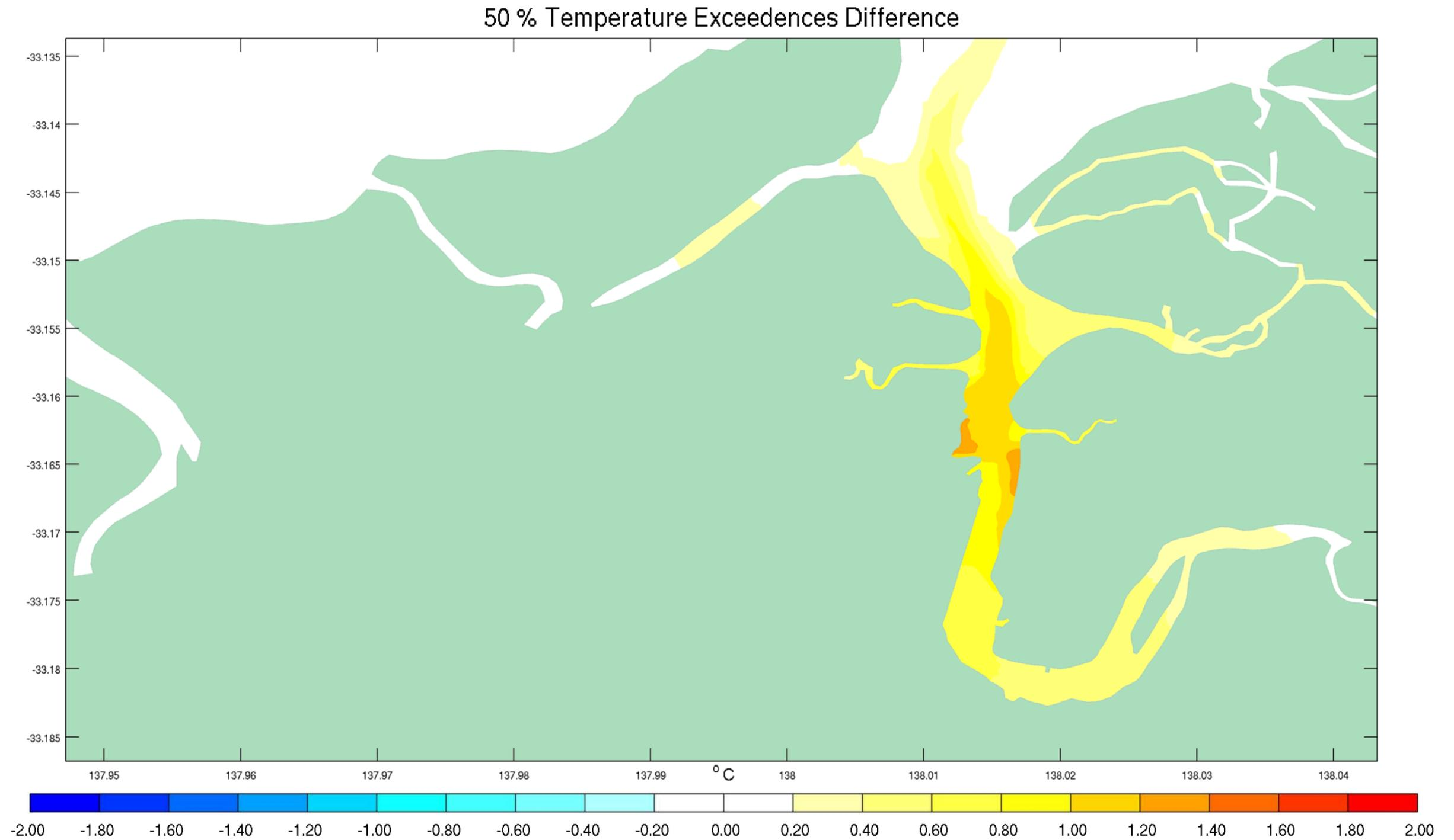
Figure E- 1250<sup>th</sup> Percentile Temperature Exceedences Difference between Discharge Scenario and Existing Conditions January to March 2013
