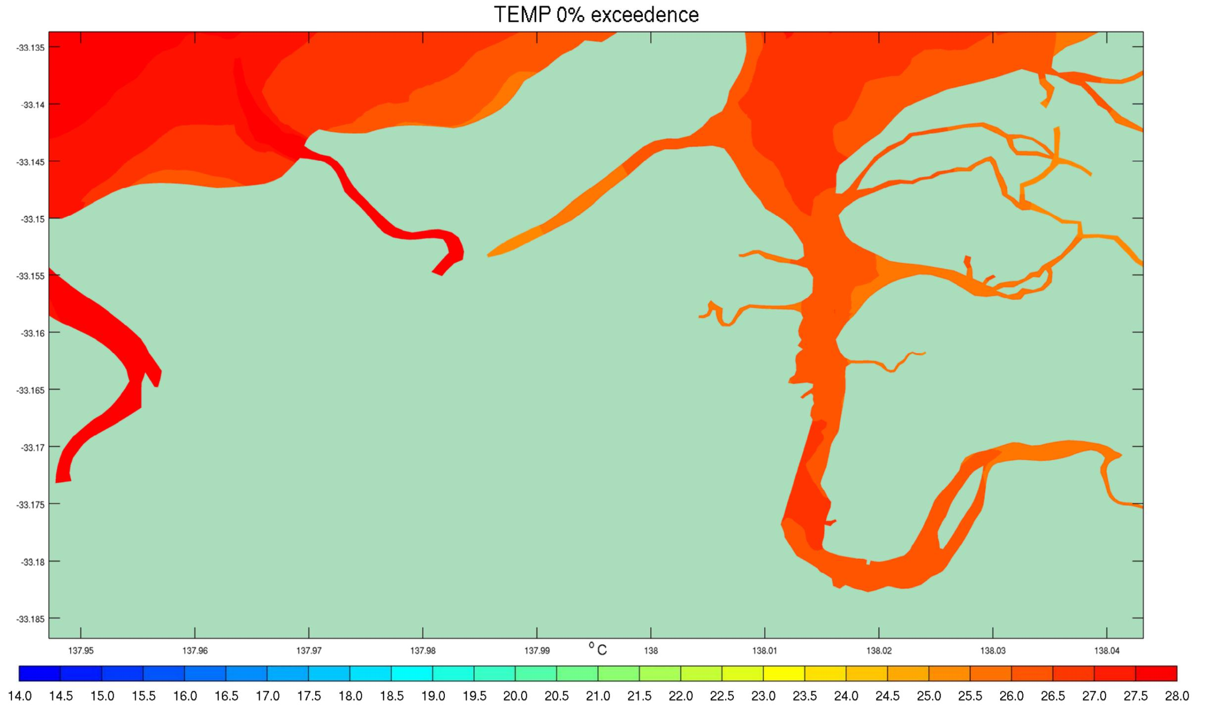
Figure A-1 0<sup>th</sup> Percentile Temperature Exceedences – Existing Conditions January 2013
