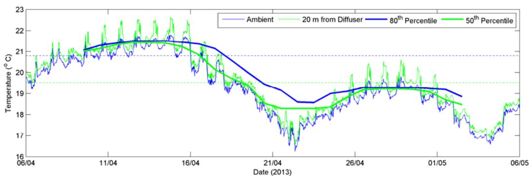
**Figure 3-5 Comparison of Ambient Temperatures (blue) and Temperatures at 20 m from Diffuser (green) for April 2013 for the Optimised Diffuser. Thick lines refer to 80<sup>th</sup> percentile ambient temperature (blue) and 50<sup>th</sup> percentile temperatures 20 m from diffuser (green) considering a 7 day period of analysis. Dashed lines refer to the analysis considering the 30 day period.**
