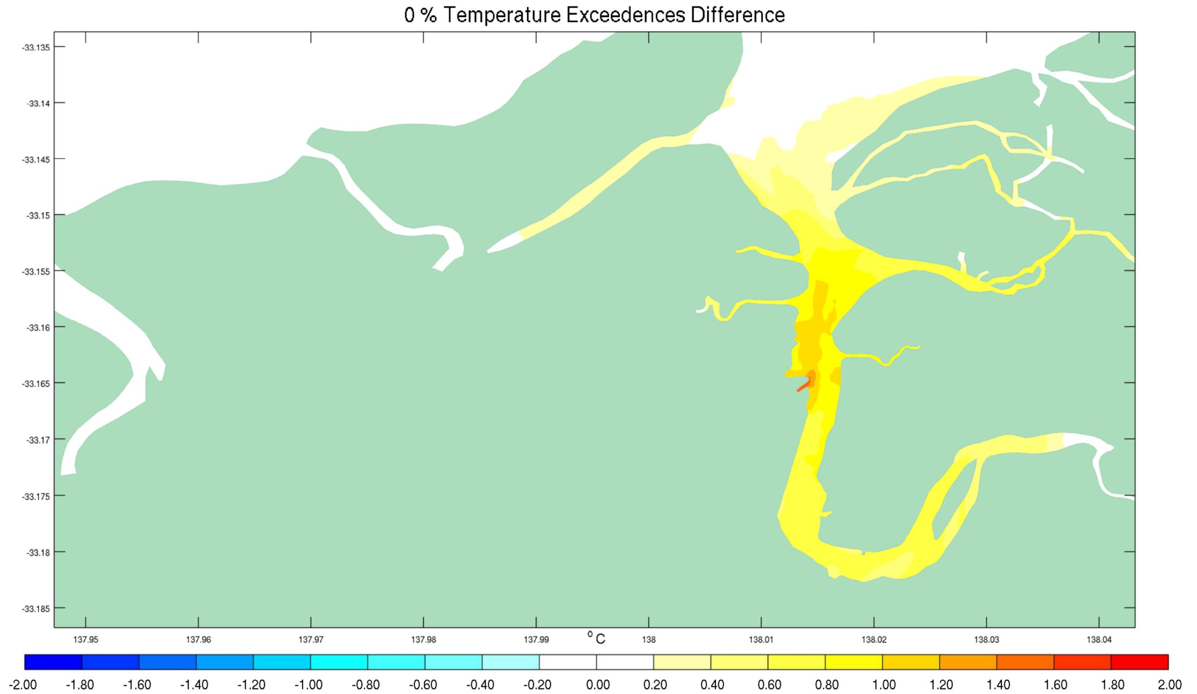
Figure E- 10 0<sup>th</sup> Percentile Temperature Exceedences Difference between Discharge Scenario and Existing Conditions January to March 2013
