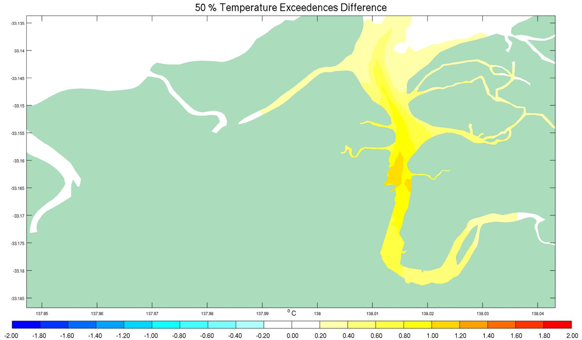
Figure F-9 50<sup>th</sup> Percentile Temperature Exceedences Difference between Discharge Scenario and Existing Conditions September 2012
