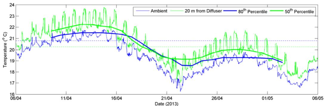
**Figure 3-4 Comparison of Ambient Temperatures (blue) and Temperatures at 20 m from Diffuser (green) for April 2013. Thick lines refer to 80<sup>th</sup> percentile ambient temperature (blue) and 50<sup>th</sup> percentile temperatures 20 m from diffuser (green) considering a 7 day period of analysis. Dashed lines refer to the analysis considering the 30 day period.**
