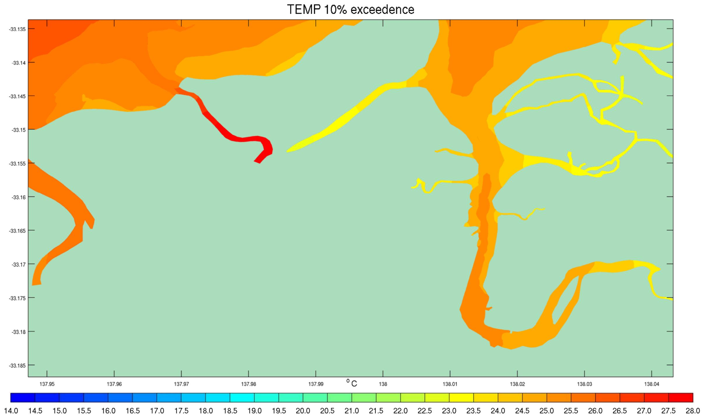
Figure 4-9 10<sup>th</sup> Percentile Temperature Exceedences – Existing Conditions February 2013
