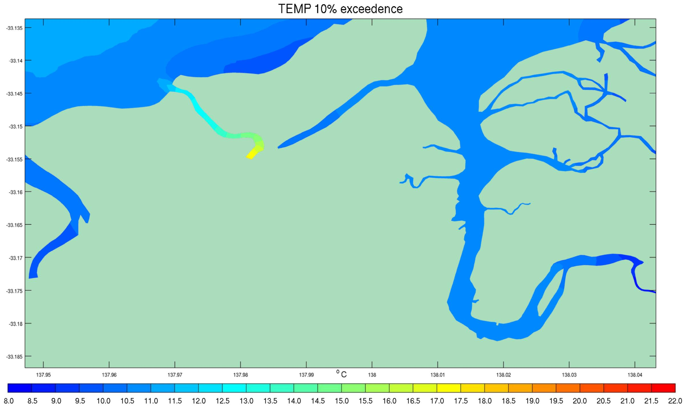
Figure 4-12 10<sup>th</sup> Percentile Temperature Exceedences – Existing Conditions July 2012
