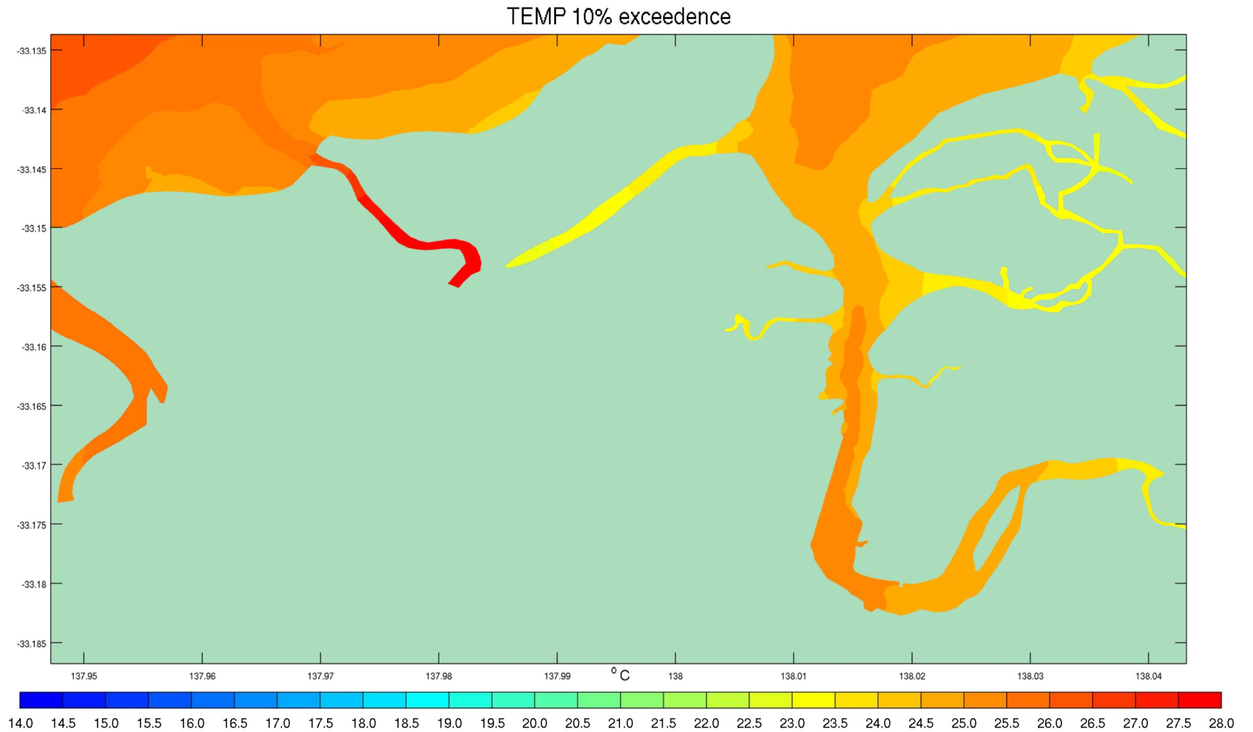
Figure A-5 10<sup>th</sup> Percentile Temperature Exceedences – Existing Conditions February 2013
