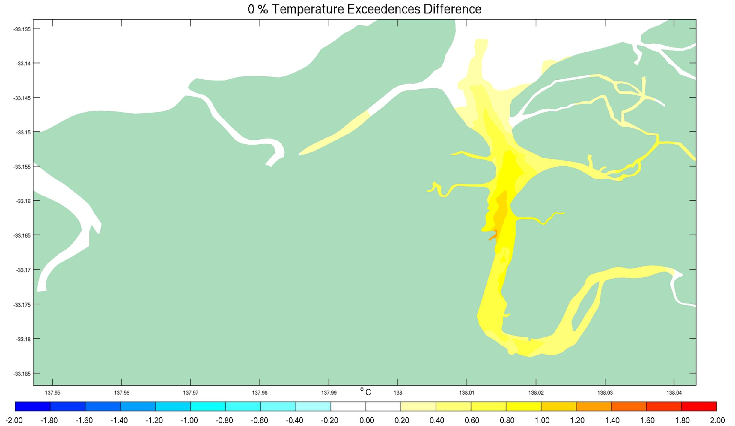
Figure E- 4 0<sup>th</sup> Percentile Temperature Exceedences Difference between Discharge Scenario and Existing Conditions February 2013
