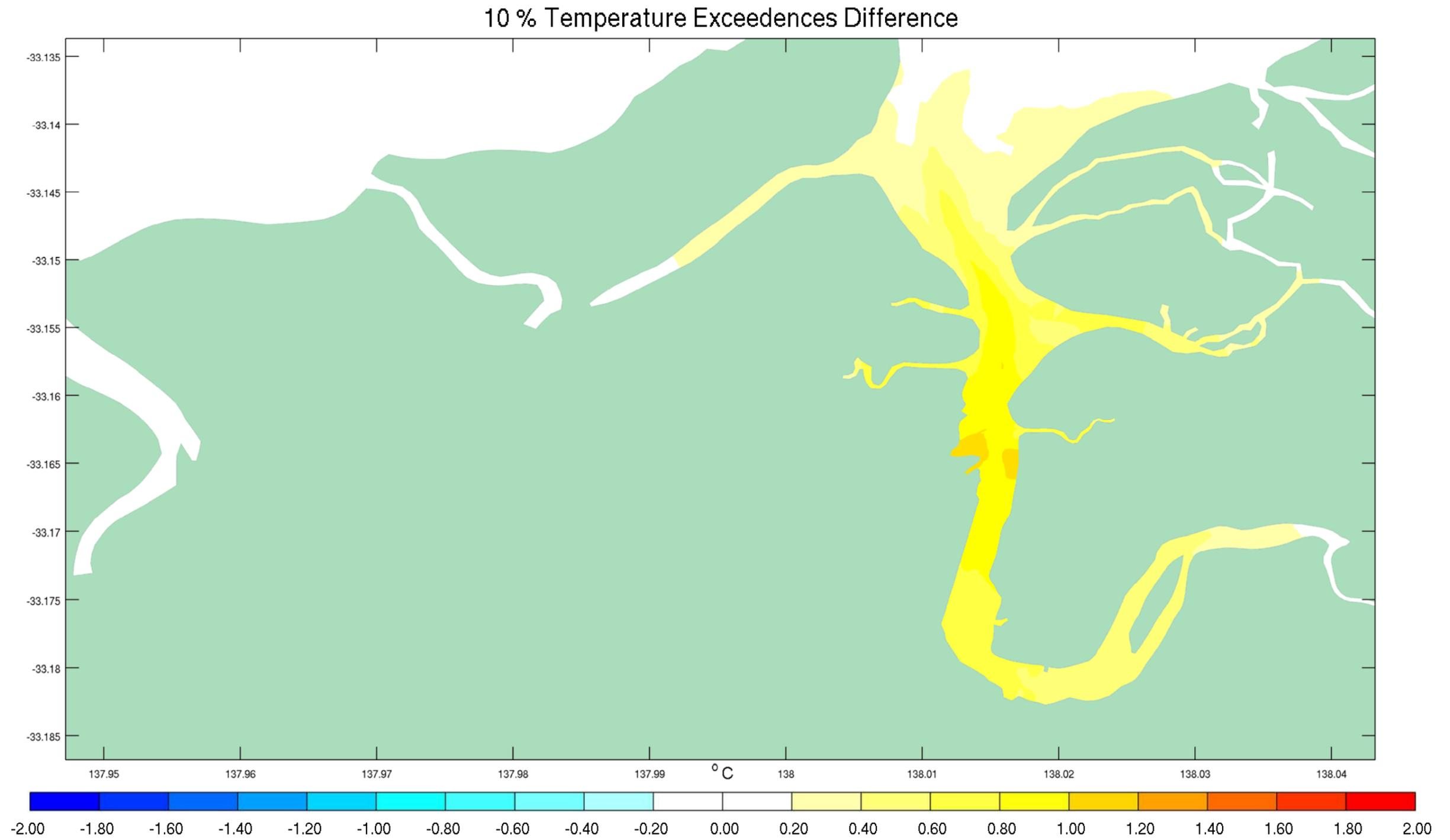
Figure E- 5 10<sup>th</sup> Percentile Temperature Exceedences Difference between Discharge Scenario and Existing Conditions February 2013
