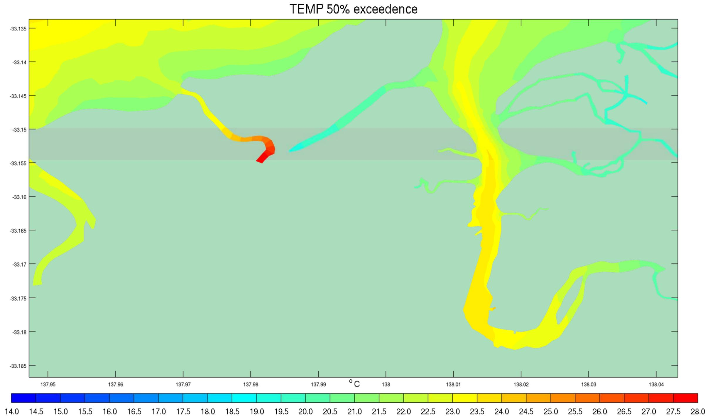
Figure C-12 50<sup>th</sup> Percentile Temperature Exceedences – Discharge Scenario Conditions January to March 2013
