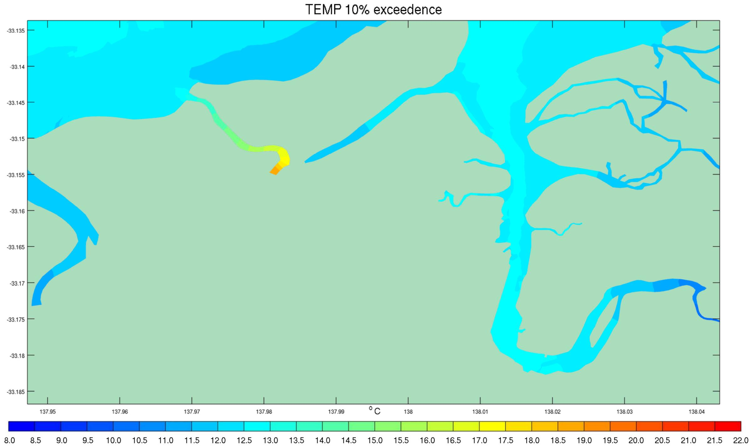
Figure 4-13 10<sup>th</sup> Percentile Temperature Exceedences – Existing Conditions August 2012
