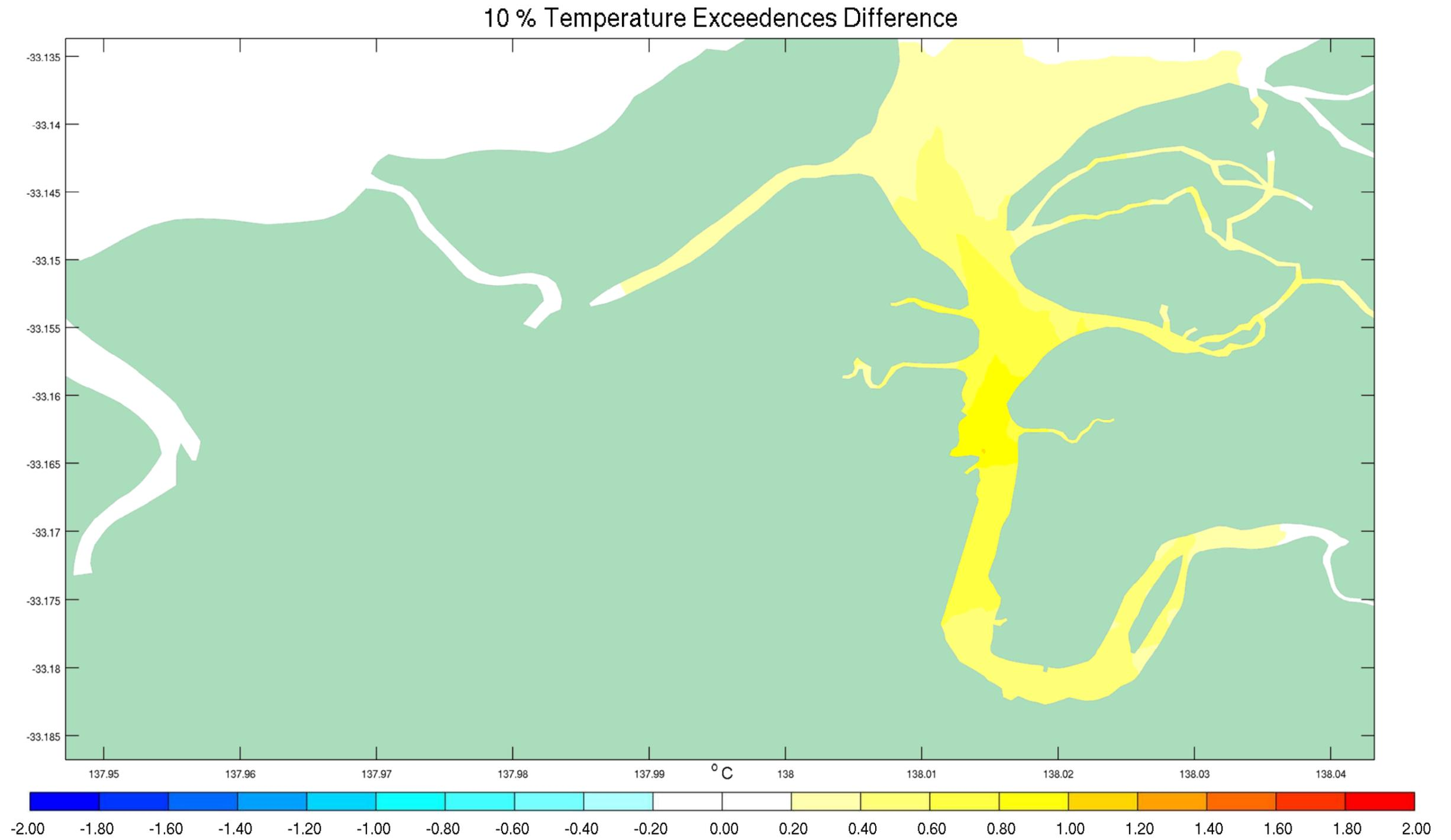
Figure F-5 10<sup>th</sup> Percentile Temperature Exceedences Difference between Discharge Scenario and Existing Conditions August 2012
