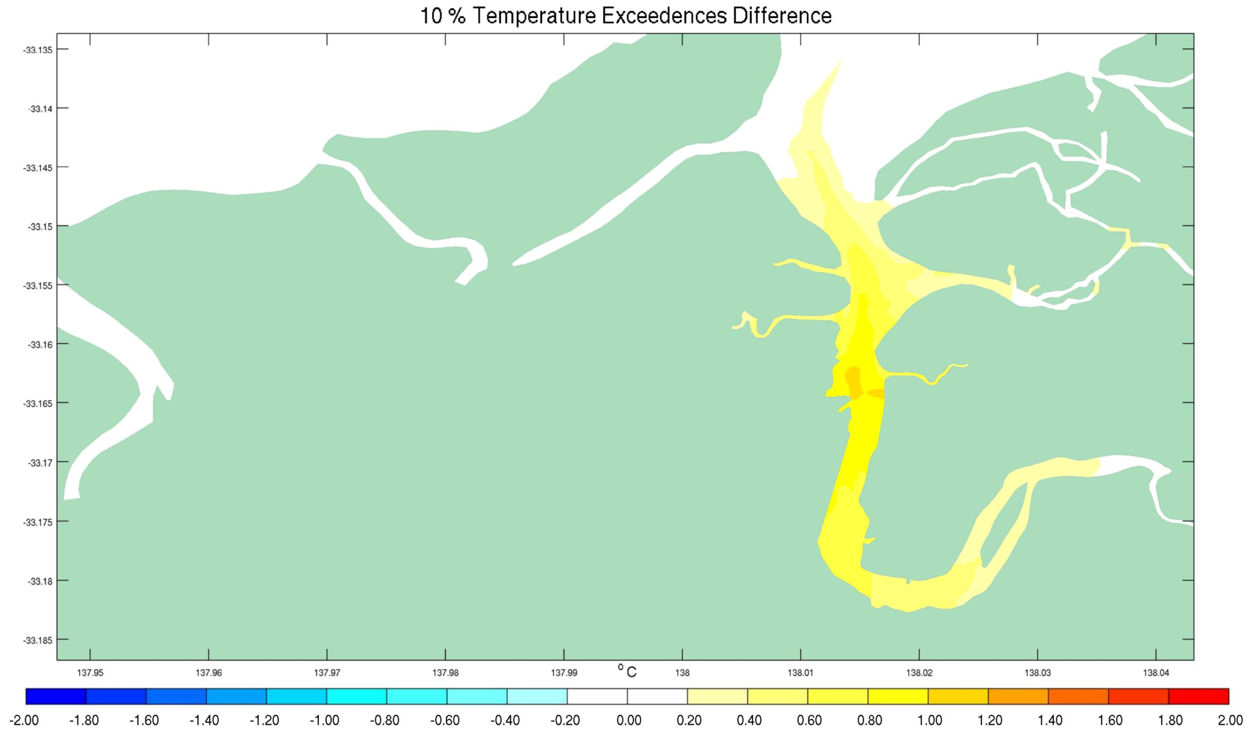
Figure E- 8 10<sup>th</sup> Percentile Temperature Exceedences Difference between Discharge Scenario and Existing Conditions March 2013
