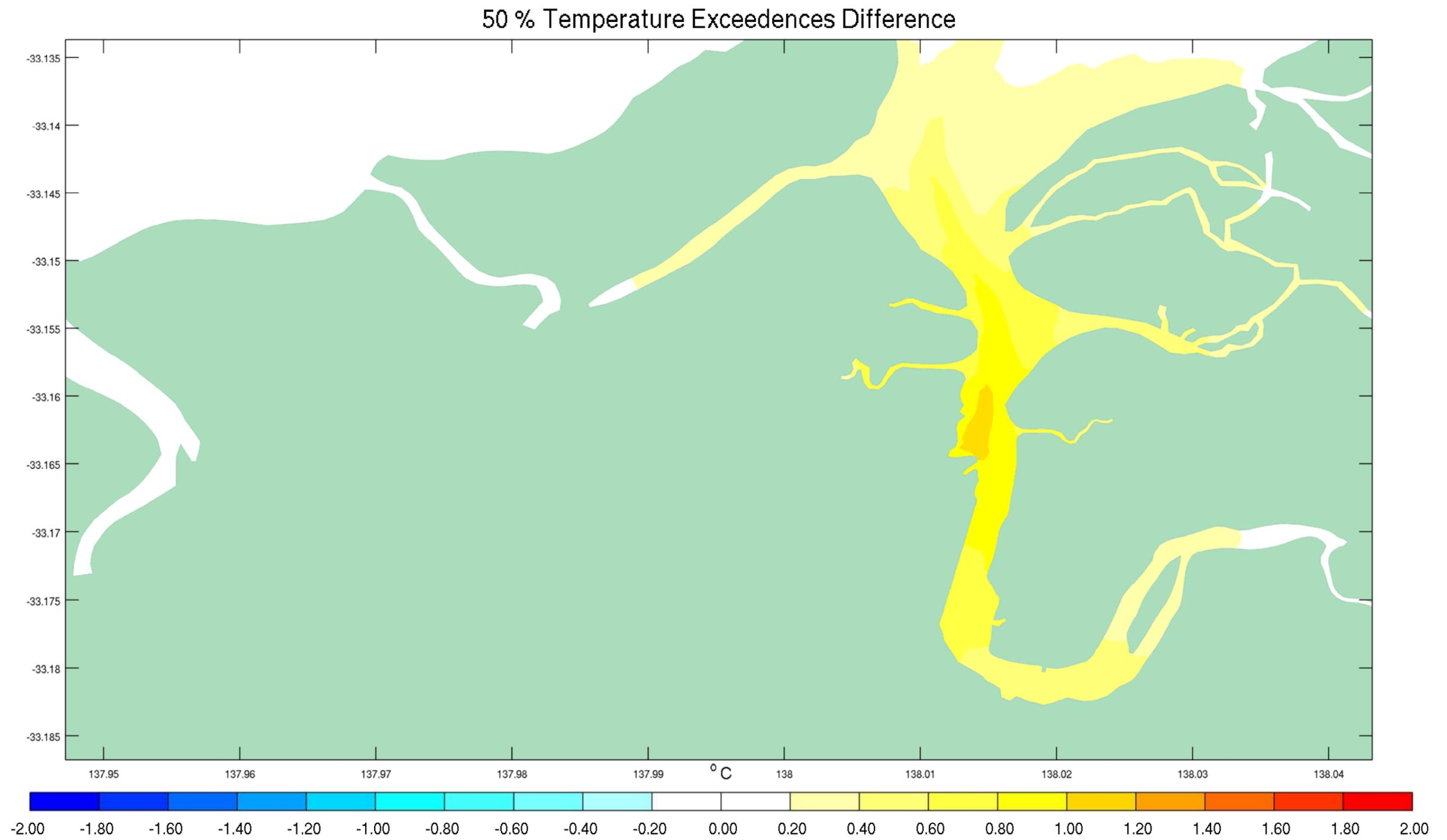
Figure F-6 50<sup>th</sup> Percentile Temperature Exceedences Difference between Discharge Scenario and Existing Conditions August 2012
