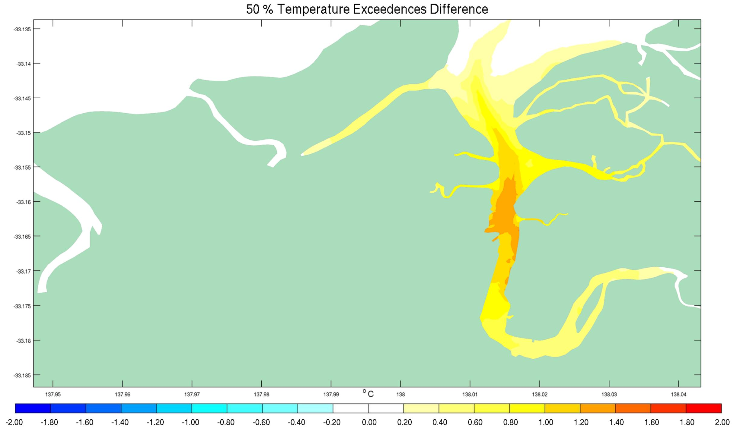
Figure E- 9 50<sup>th</sup> Percentile Temperature Exceedences Difference between Discharge Scenario and Existing Conditions March 2013
