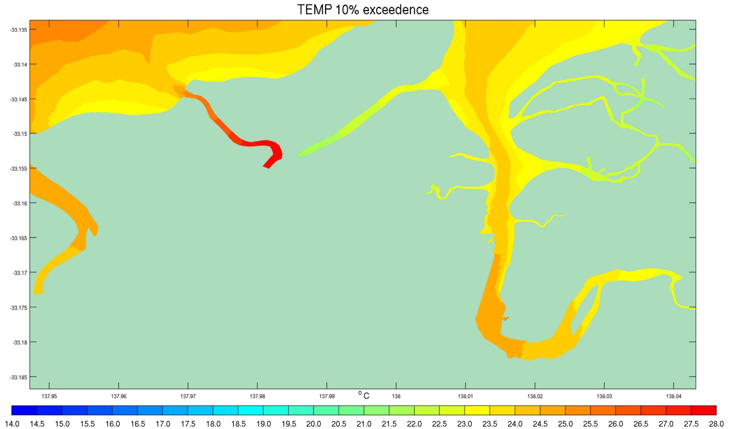
Figure A- 2 10<sup>th</sup> Percentile Temperature Exceedences – Existing Conditions January 2013
