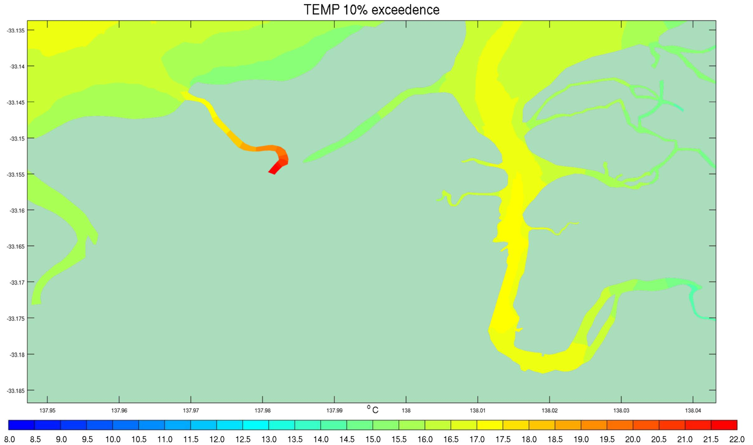
Figure 4-22 10<sup>th</sup> Percentile Temperature Exceedences – Discharge Scenario Conditions September 2012
