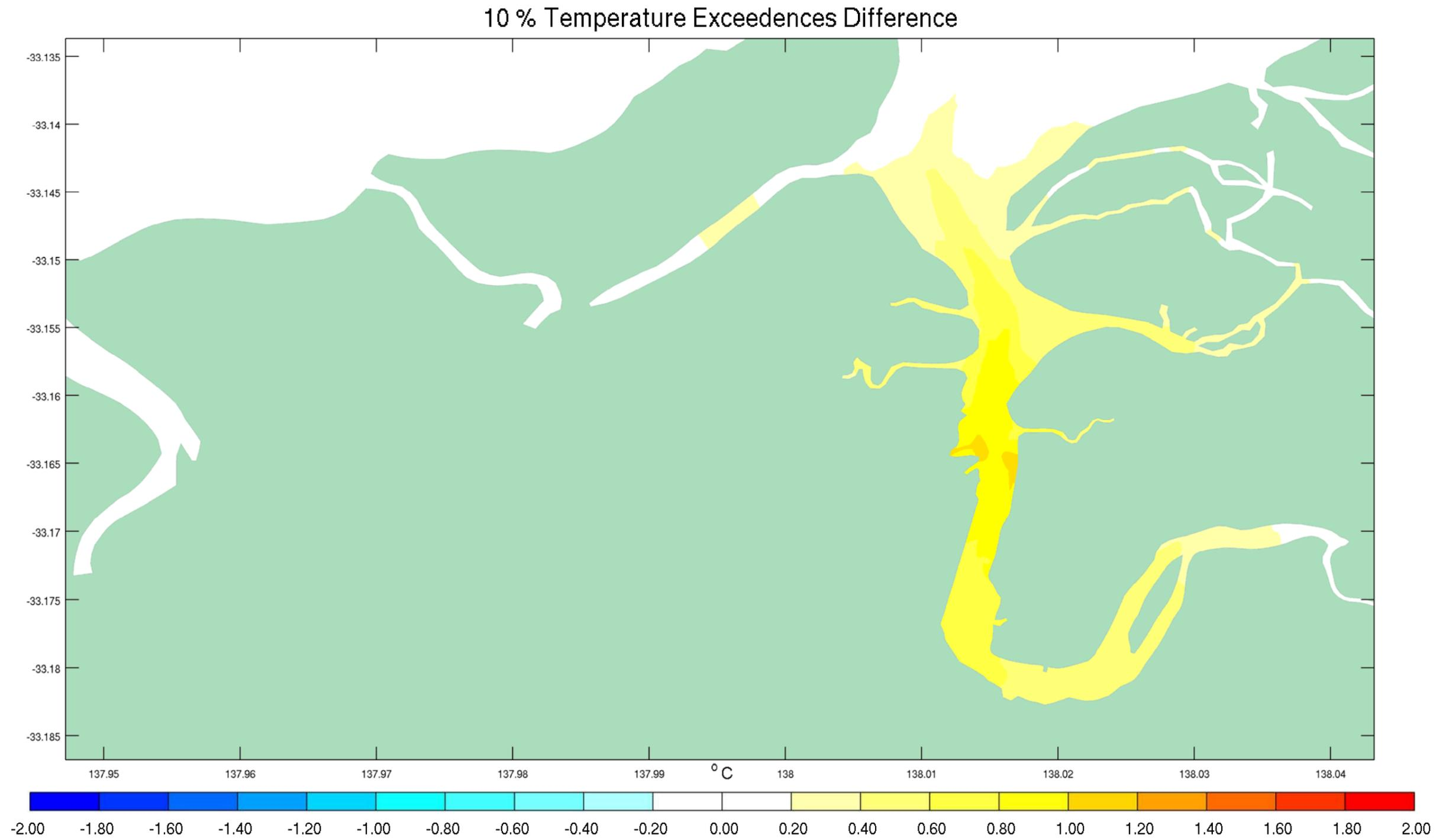
Figure E- 11 10<sup>th</sup> Percentile Temperature Exceedences Difference between Discharge Scenario and Existing Conditions January to March 2013
