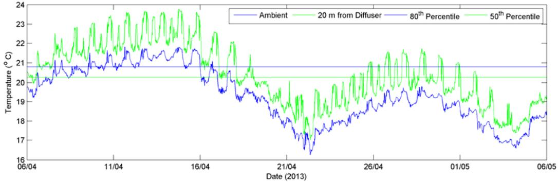
**Figure 3-3 Comparison of Ambient Temperatures (blue) and Temperatures at 20 m from Diffuser (green) for April 2013. Straight Lines refer to 80<sup>th</sup> percentile ambient temperature (blue) and 50<sup>th</sup> percentile temperatures 20 m from diffuser (green) considering a one month period of analysis as per BMT WBM (2013).**
