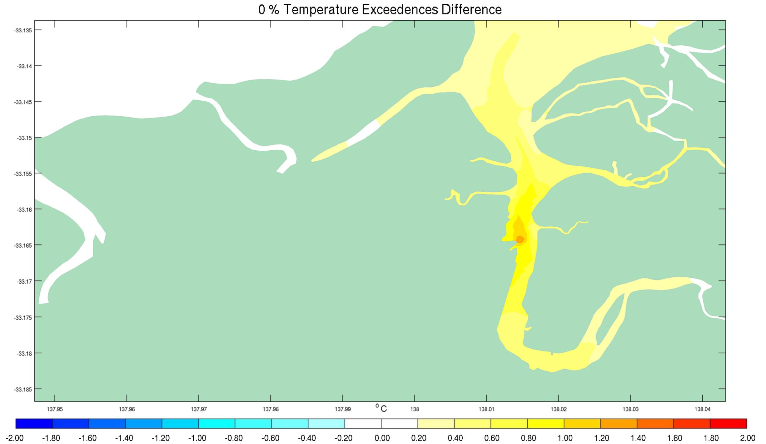
Figure F-4 0<sup>th</sup> Percentile Temperature Exceedences Difference between Discharge Scenario and Existing Conditions August 2012
