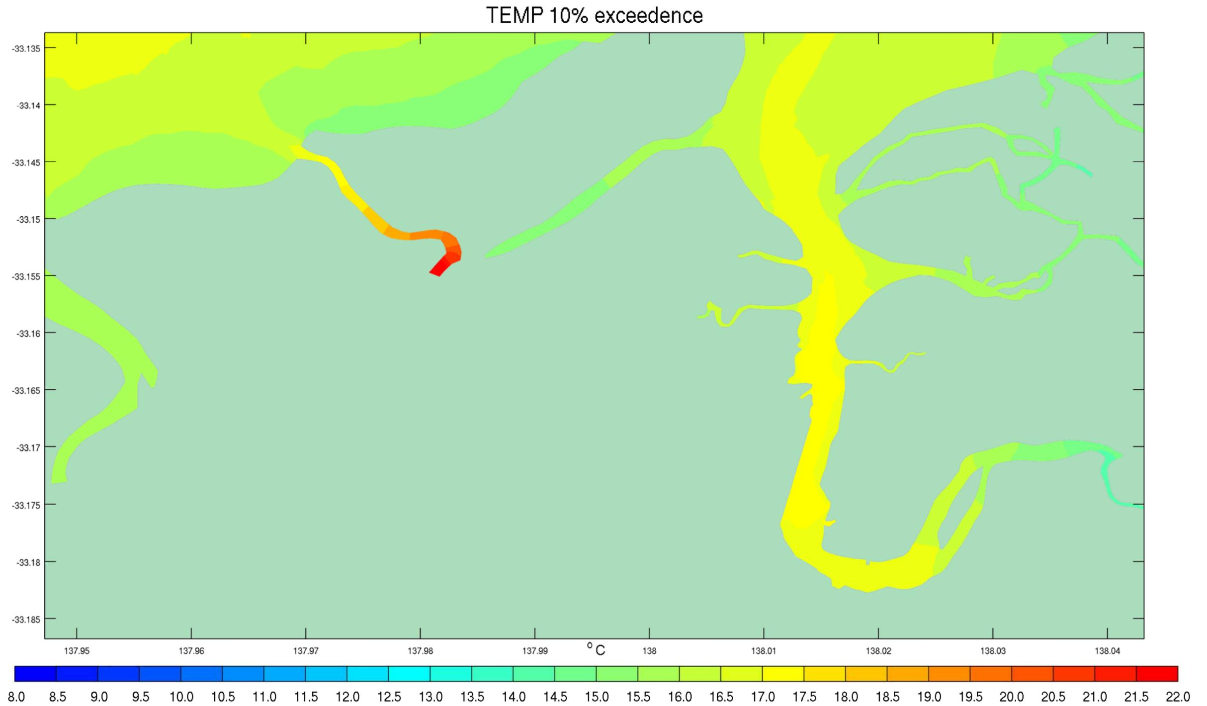
Figure D- 8 10<sup>th</sup> Percentile Temperature Exceedences – Discharge Scenario Conditions September 2012
