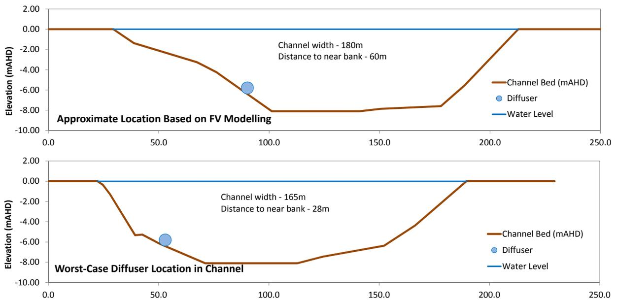
Figure 3-2 Nominal and Worst-Case Channel Cross Sectional Geometry
