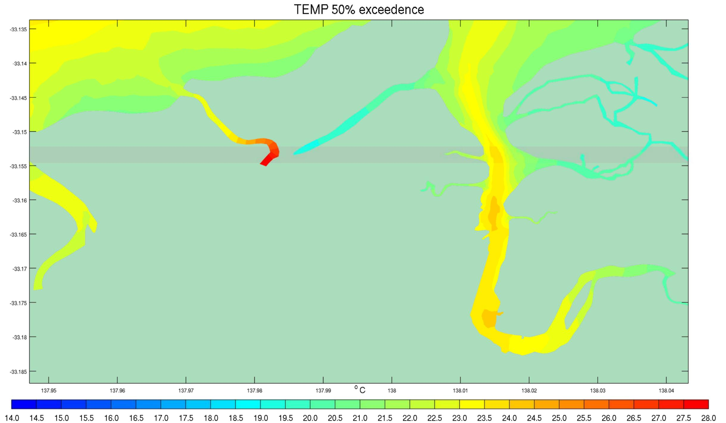
Figure C-3 50<sup>th</sup> Percentile Temperature Exceedences – Discharge Scenario Conditions January 2013
