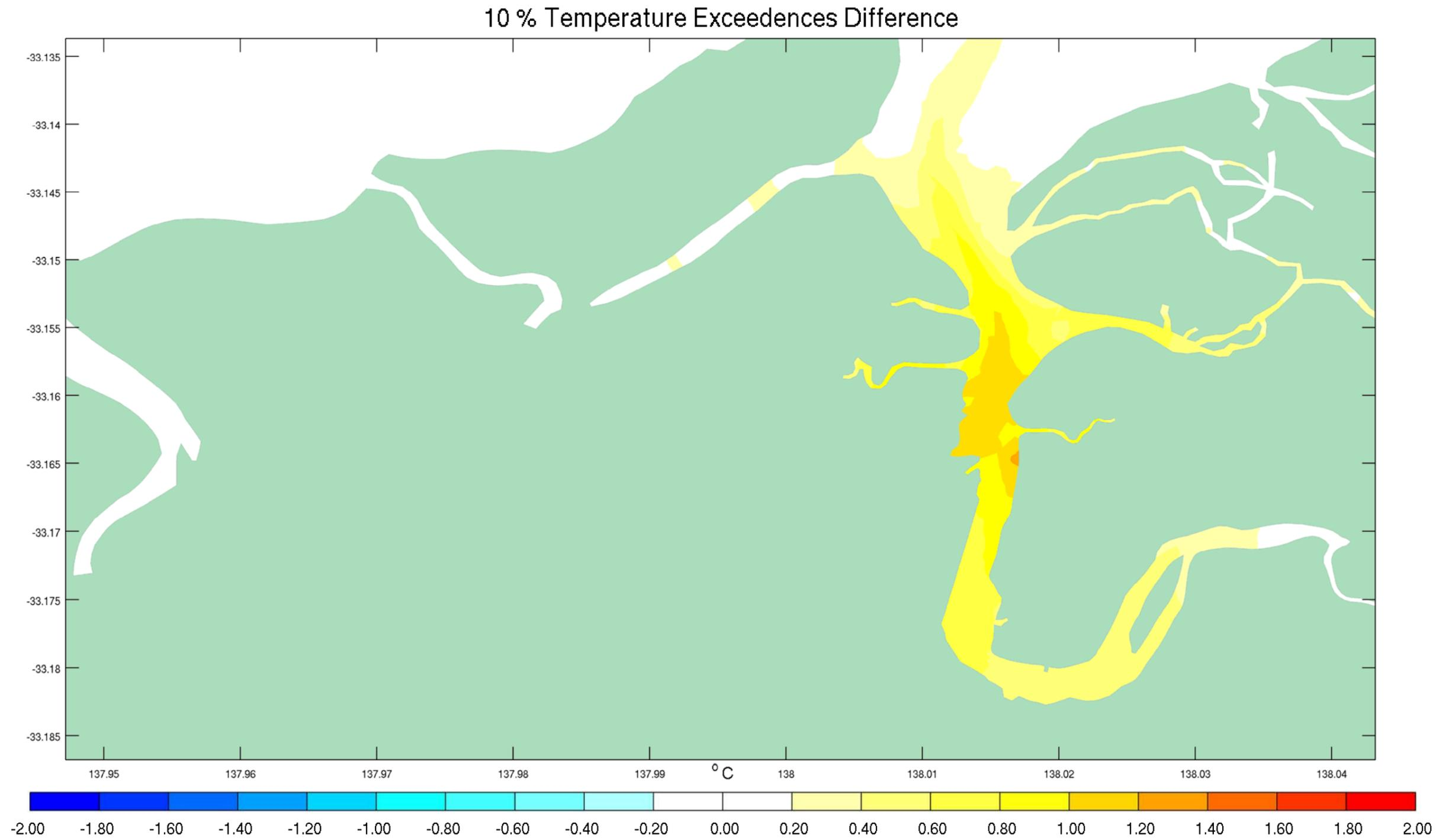
Figure E- 2 10<sup>th</sup> Percentile Temperature Exceedences Difference between Discharge Scenario and Existing Conditions January 2013
