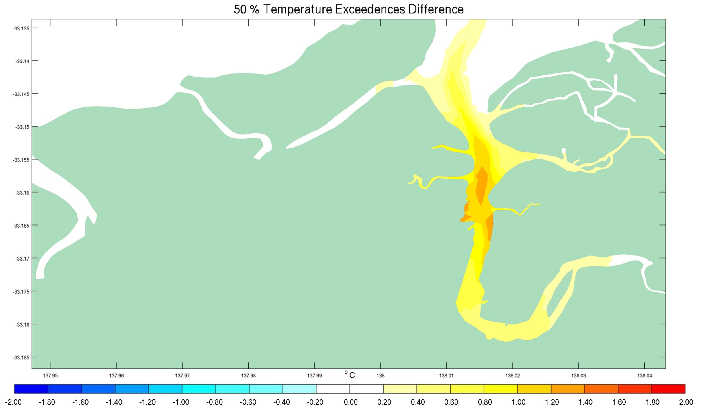
Figure E- 3 50<sup>th</sup> Percentile Temperature Exceedences Difference between Discharge Scenario and Existing Conditions January 2013
