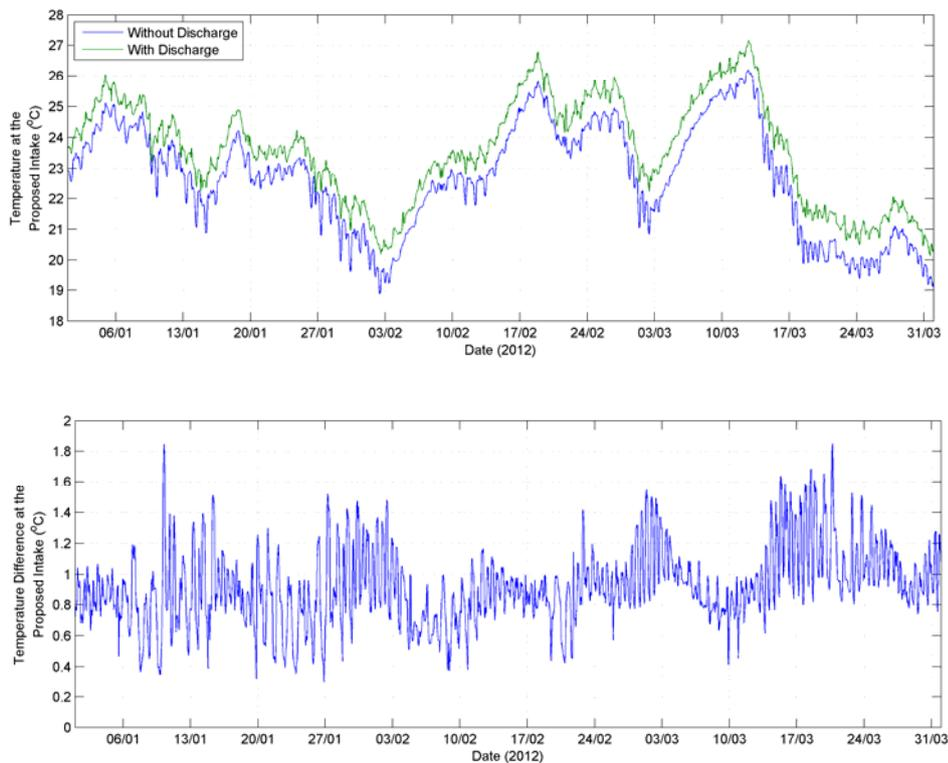
**Figure 4-32 Upper Panel: Temperature at the Location of the Proposed Intake for Summer Simulations. Lower Panel: Temperature Difference between Discharge Scenario and Baseline at the Location of the Proposed Intake for Summer Simulations**
