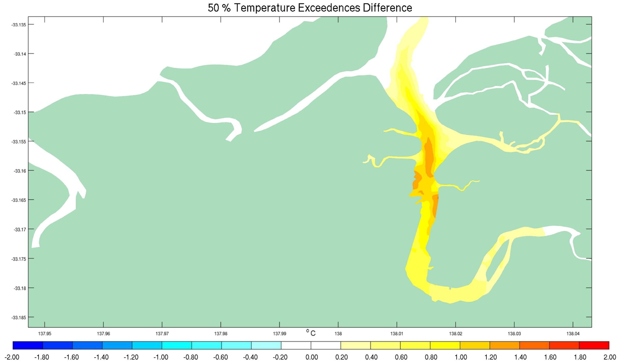
Figure E- 6 50<sup>th</sup> Percentile Temperature Exceedences Difference between Discharge Scenario and Existing Conditions February 2013
