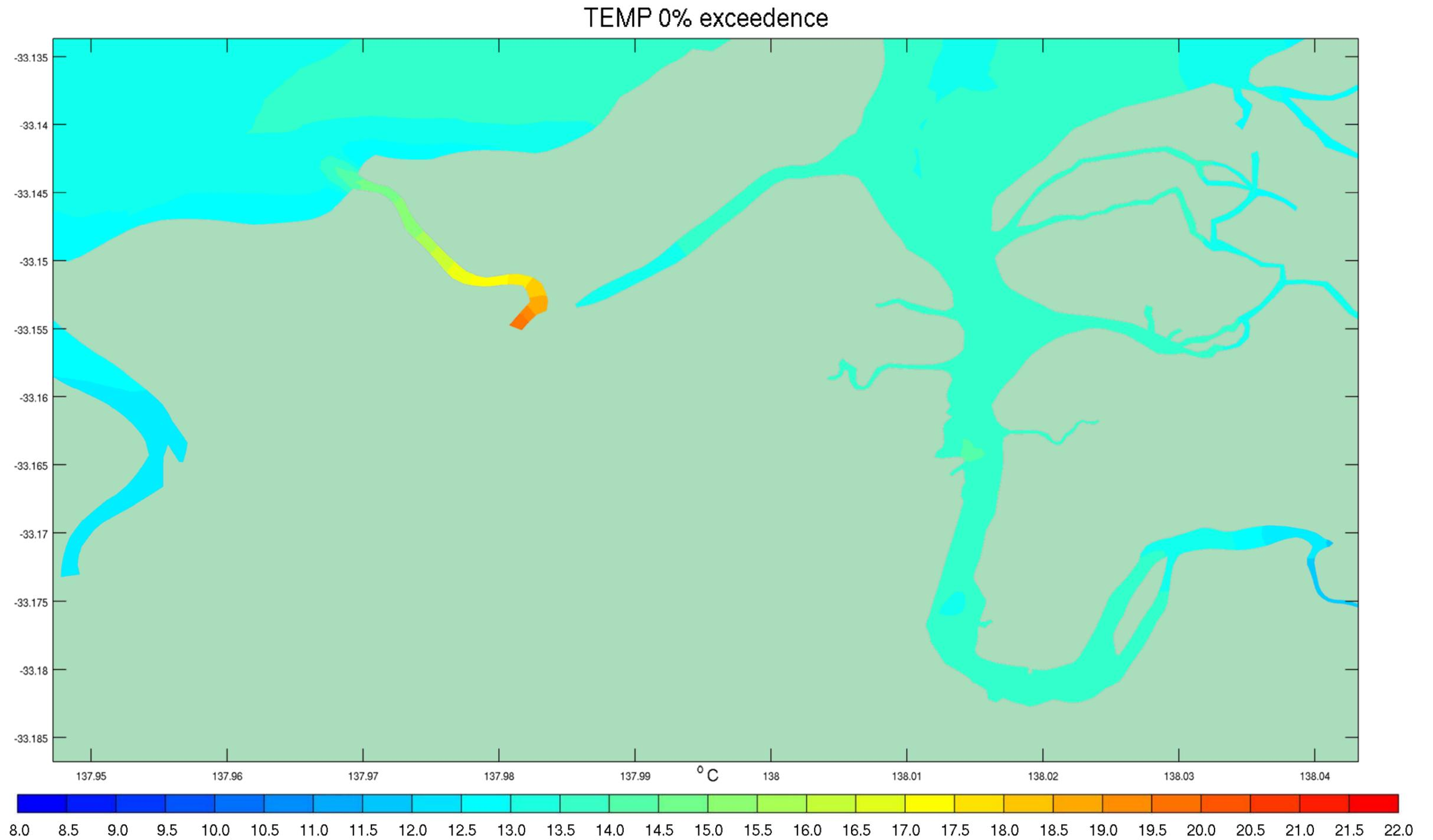
Figure D- 4 0<sup>th</sup> Percentile Temperature Exceedences – Discharge Scenario Conditions August 2012
