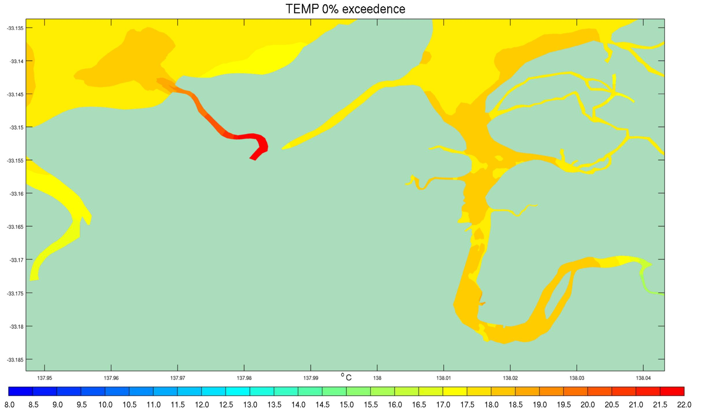
Figure D- 10 0<sup>th</sup> Percentile Temperature Exceedences – Discharge Scenario Conditions July to September 2012
