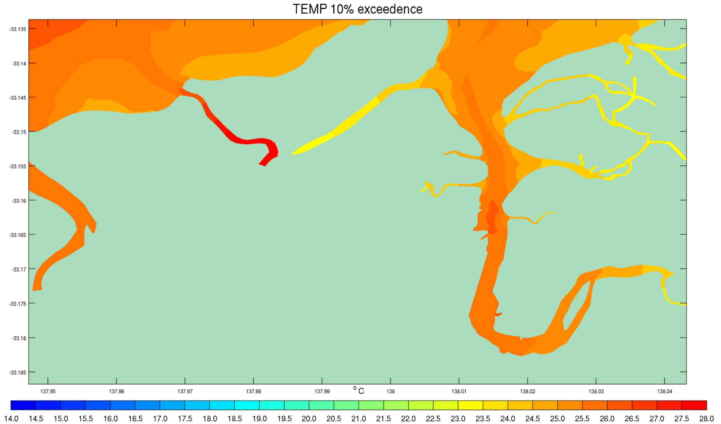
Figure 4-19 10<sup>th</sup> Percentile Temperature Exceedences – Discharge Scenario Conditions January to March 2013
