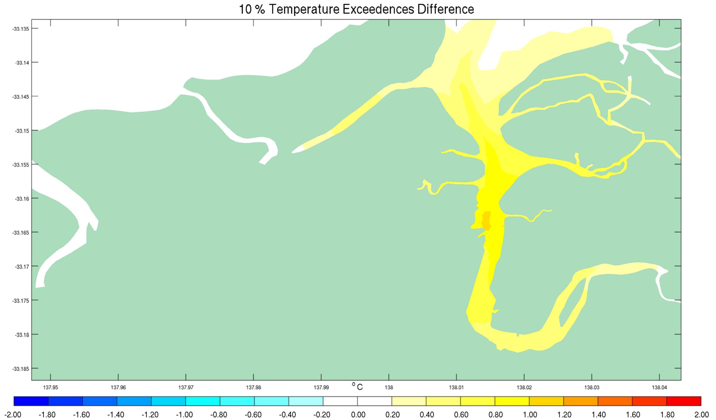
Figure 4-28 10<sup>th</sup> Percentile Temperature Exceedences Differences - July 2012
