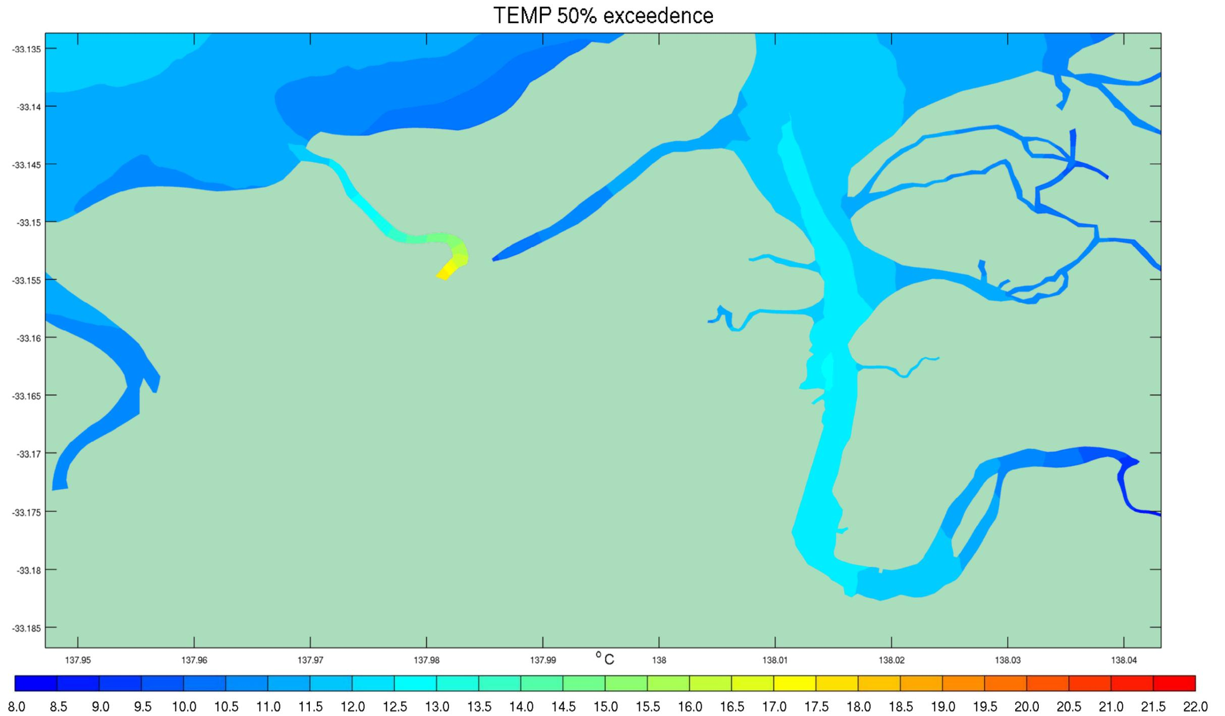
Figure D- 12 50<sup>th</sup> Percentile Temperature Exceedences – Discharge Scenario Conditions July to September 2012
