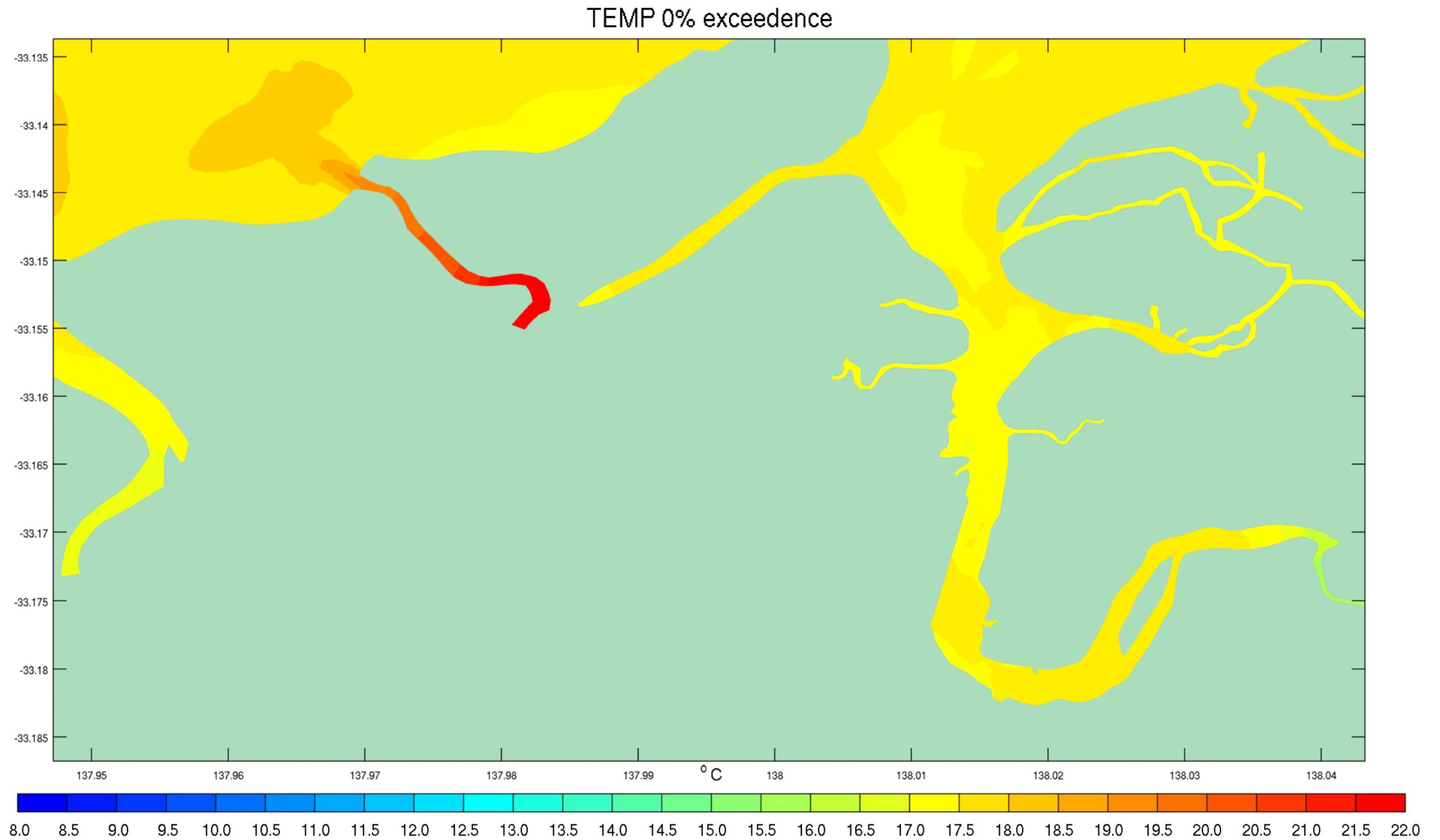
Figure B-7 0<sup>th</sup> Percentile Temperature Exceedences – Existing Conditions September 2012
