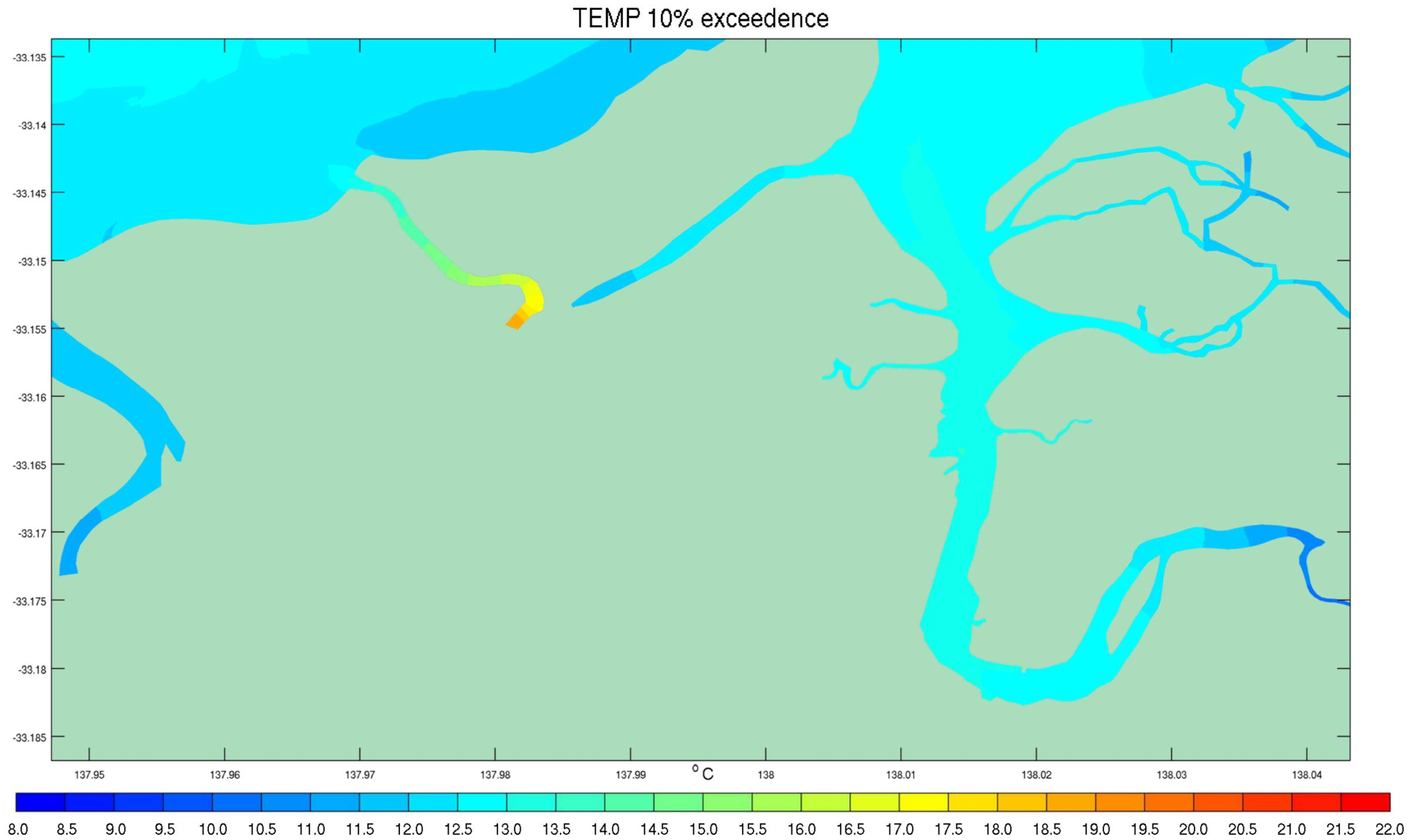
Figure 4-21 10<sup>th</sup> Percentile Temperature Exceedences – Discharge Scenario Conditions August 2012
