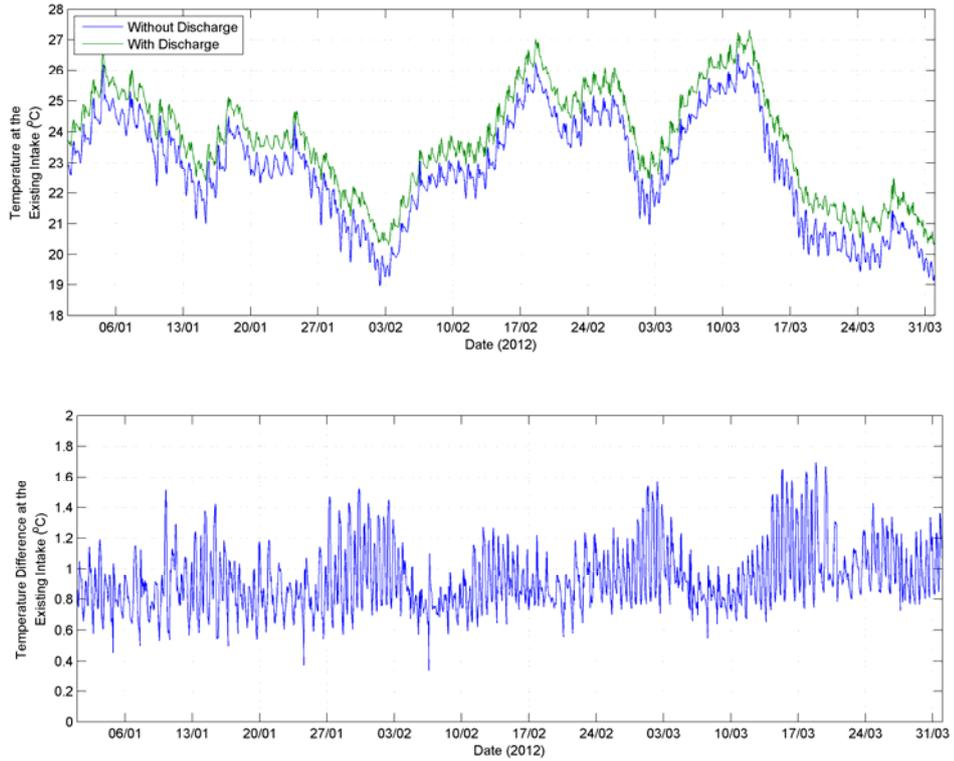
**Figure 4-33 Upper Panel: Temperature at the Location of the Existing Intake for Summer Simulations. Lower Panel: Temperature Difference between Discharge Scenario and Baseline at the Location of the Existing Intake for Summer Simulations.**
