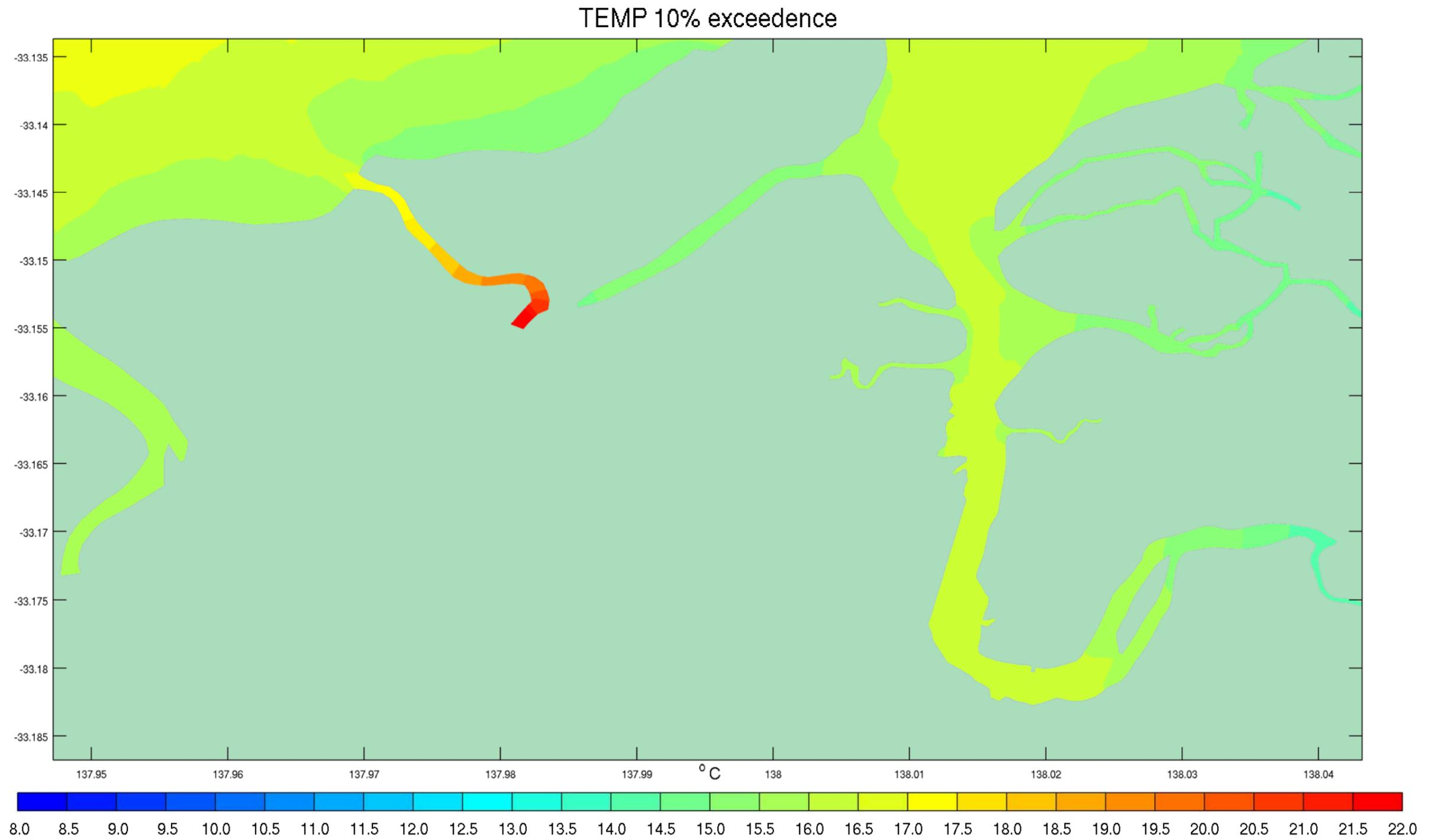
Figure B- 8 10<sup>th</sup> Percentile Temperature Exceedences – Existing Conditions September 2012
