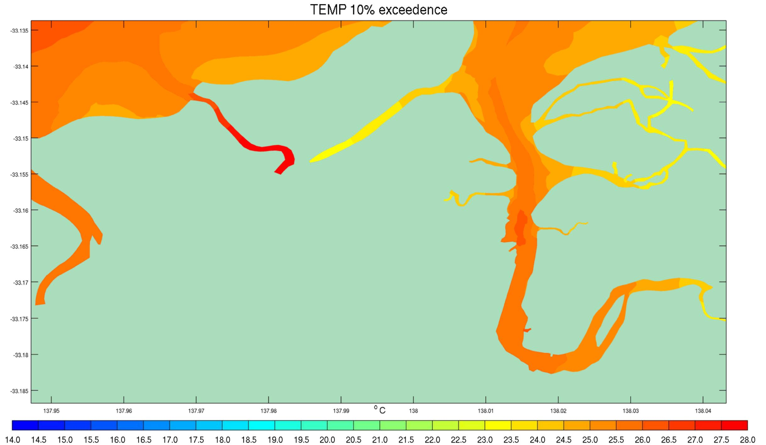
Figure C-11 10<sup>th</sup> Percentile Temperature Exceedences – Discharge Scenario Conditions January to March 2013
