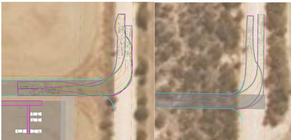
Figure 6: 19.0 m semi-trailers entering and exiting the site at the proposed access points
