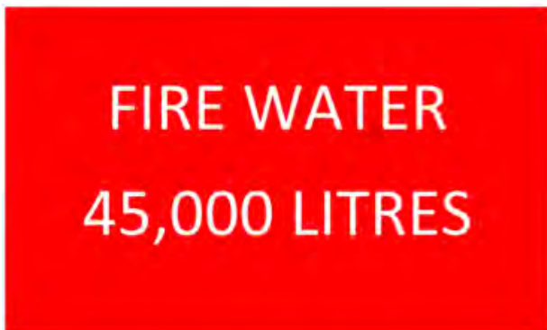
Figure 5: Fire water signage to comply with AS 2419.1-2021, Clause 11.3.6: Water storage tanks and equipment.
