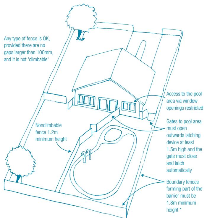
\* Boundary fences forming part of the barrier must be 1.8m high, with a 900mm non-climbable zone at the top on the pool side of the fence.
