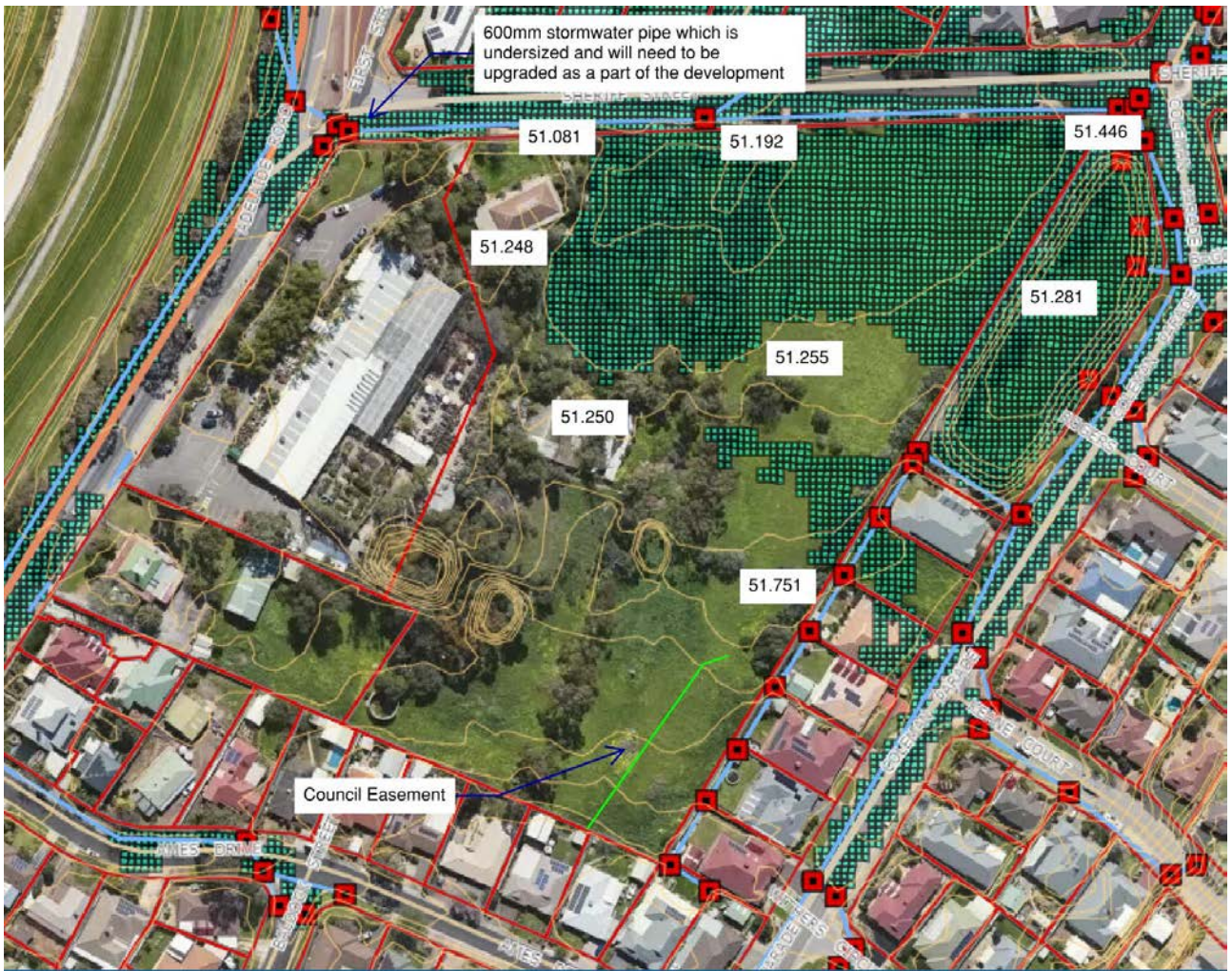
Figure 3-Council Flood Map/Stormwater network
