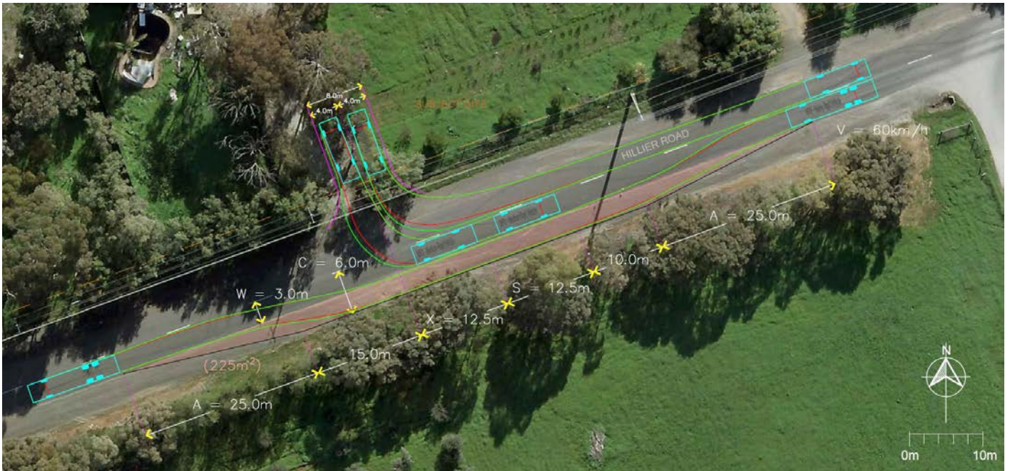
Figure 7: Indicative site access point location and arrangement with simultaneous MRV site accessibility
