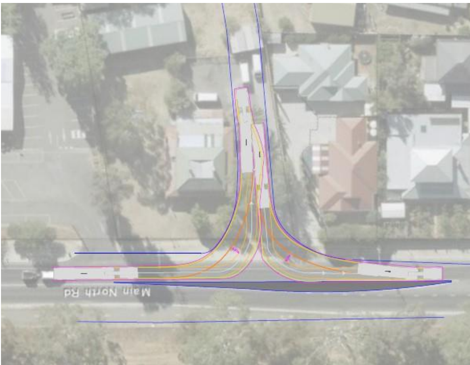
Figure 2: Commercial vehicle access
