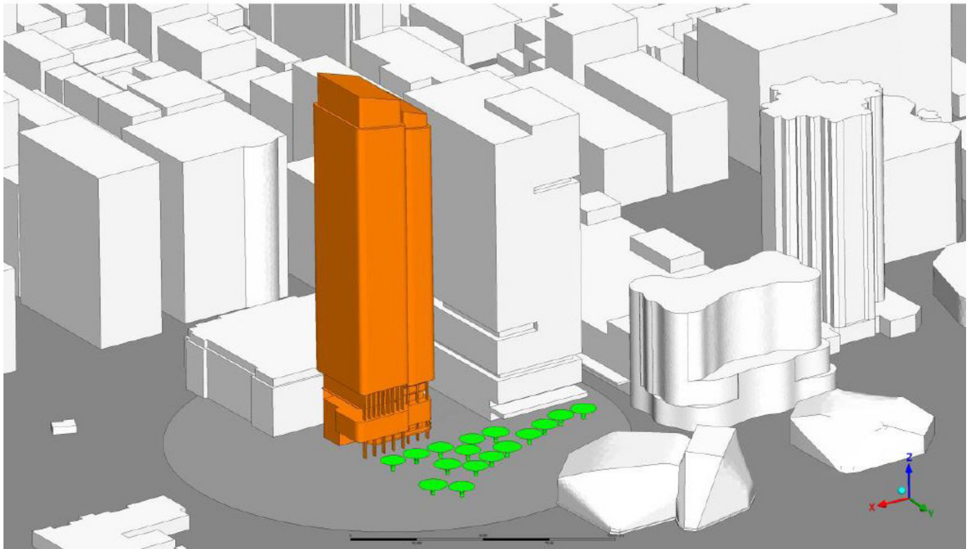
Figure 7: CFD model geometry – northeast close-up view of Walker development (Configuration 3).
