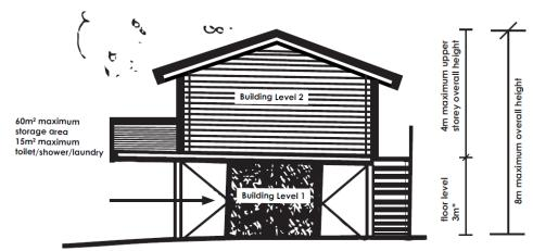
\*3m maximum finished floor level height (unless demonstrated need for higher level to mitigate against 1% AEP flood event, and in such cases then not exceeding 4m in height). Better guidance on design techniques and building materials for underfloor areas
