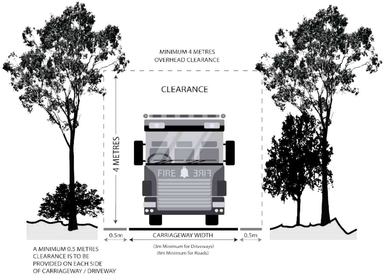
Figure 1 - Overhead and Side Clearances
