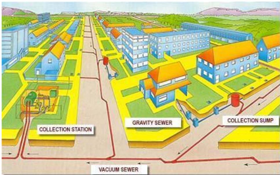
**Fig 3.2 Typical Scheme Layout**
