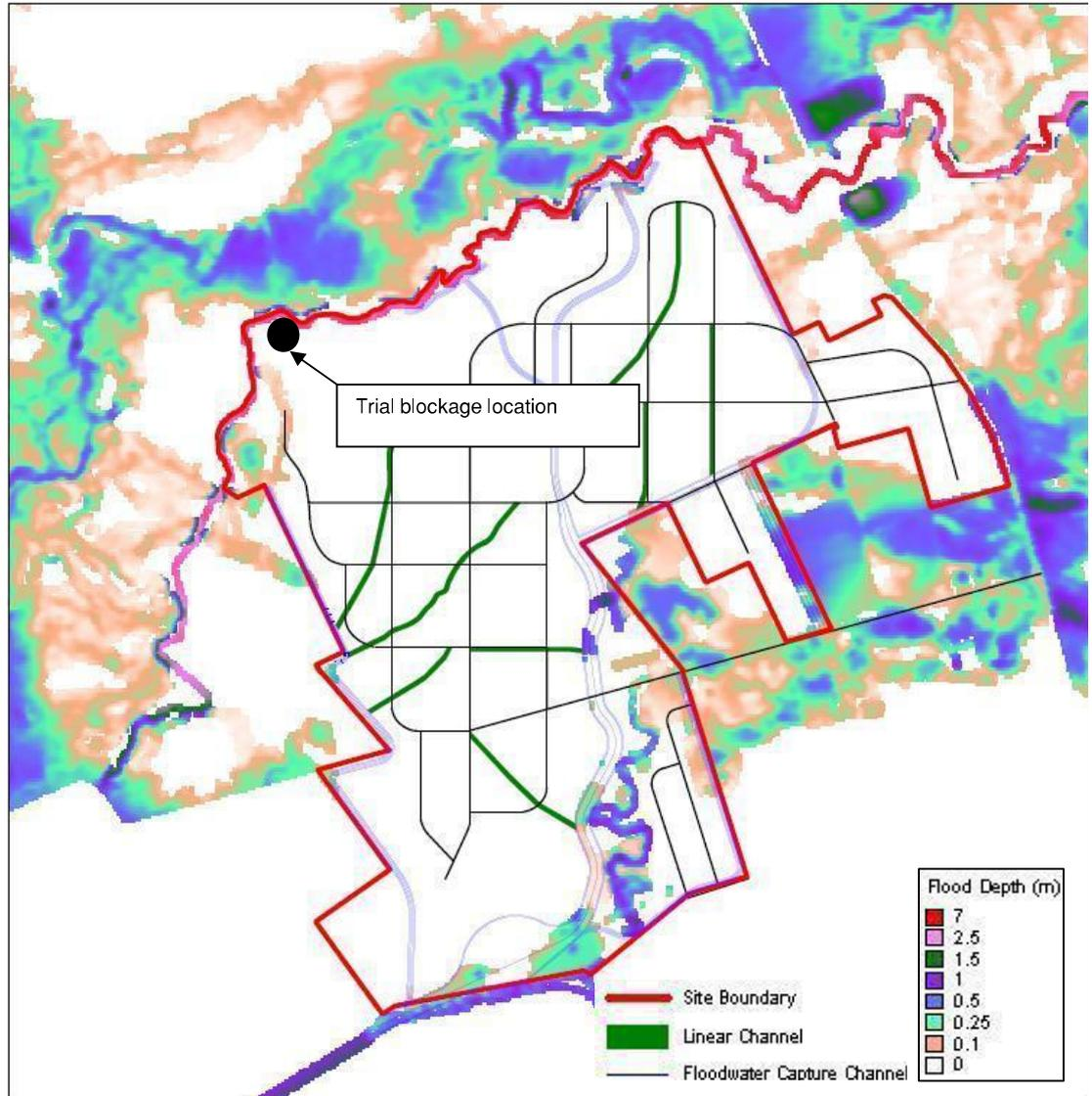
Figure 4.8 - 100 year ARI floodplain with a 25 percent blockage of Gawler River at Location 2
