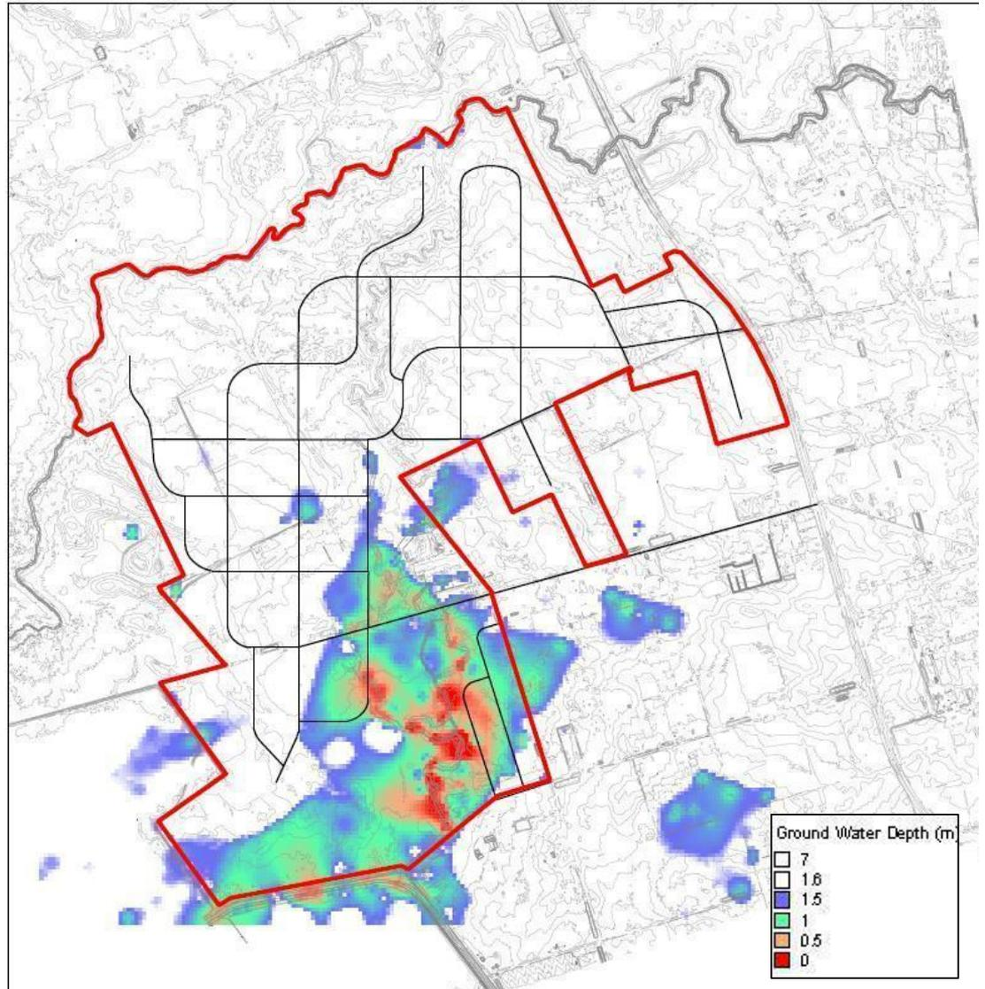
Figure 5.2 - Depth to Groundwater within 1.5m of existing surface level.
