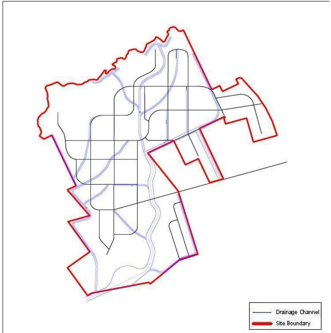
**Figure 2.3 – Proposed Lineal Open Drainage System**
