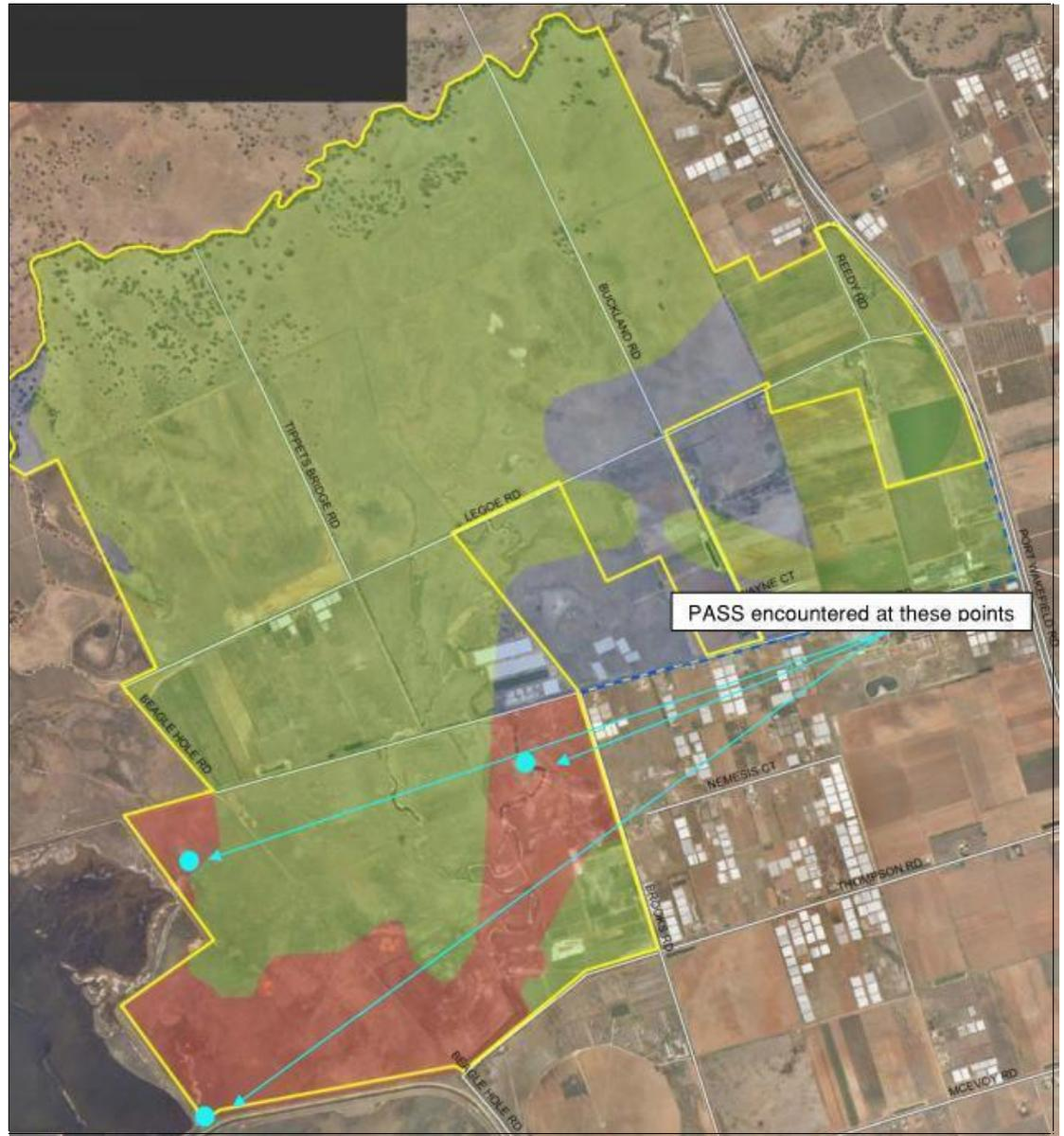
Figure 5.3 - Potential acid sulphate soil locations.
