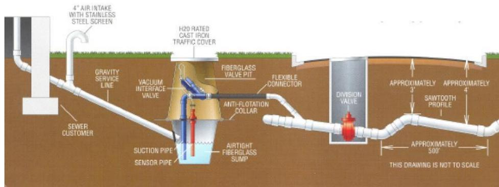
**Figure 3.3 Saw-tooth Design**
