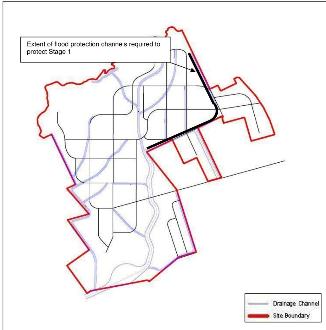
Figure 8.4 - Stage 1 – Flood Mitigation Channel Requirements
