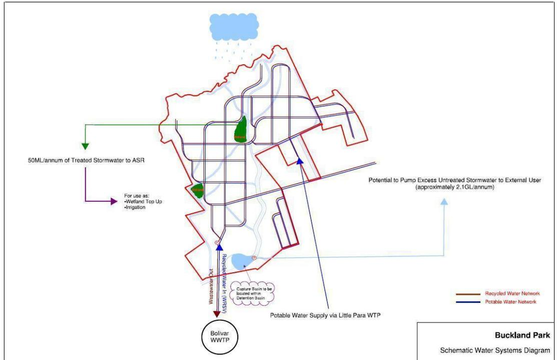
Figure 6.1 Buckland Park Water and Recycled Water Supply Schematic
