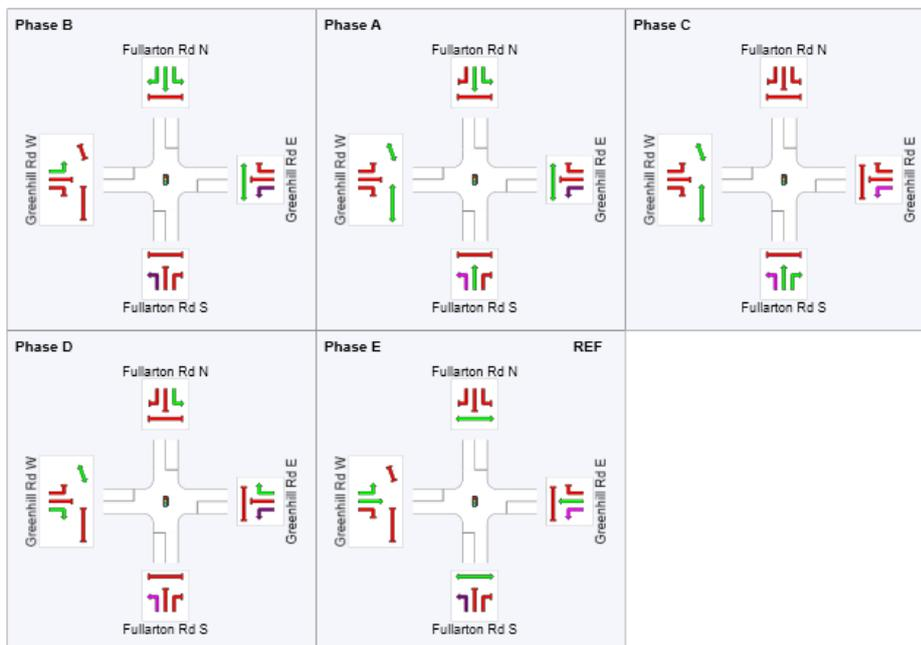
**Figure 6: SCATS Extracted Phase Sequence – TS070**
