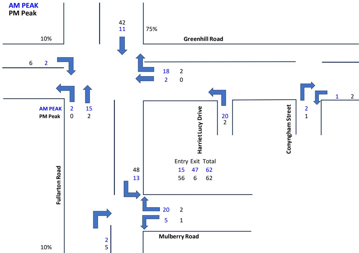
**Figure 5 Forecast Distribution of Additional AM and PM Peak Hour Movements.**
