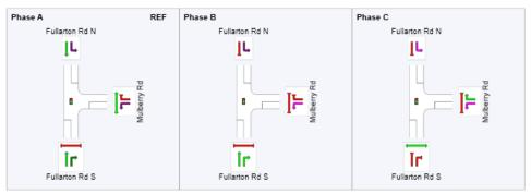
Figure 7 SIDRA Phase Sequence – TS577
