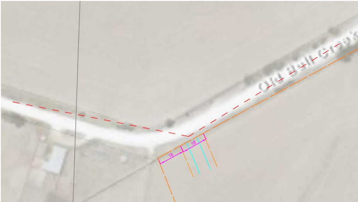
Figure 3: SISD requirement at western intersection (50 km/h speed limit)
